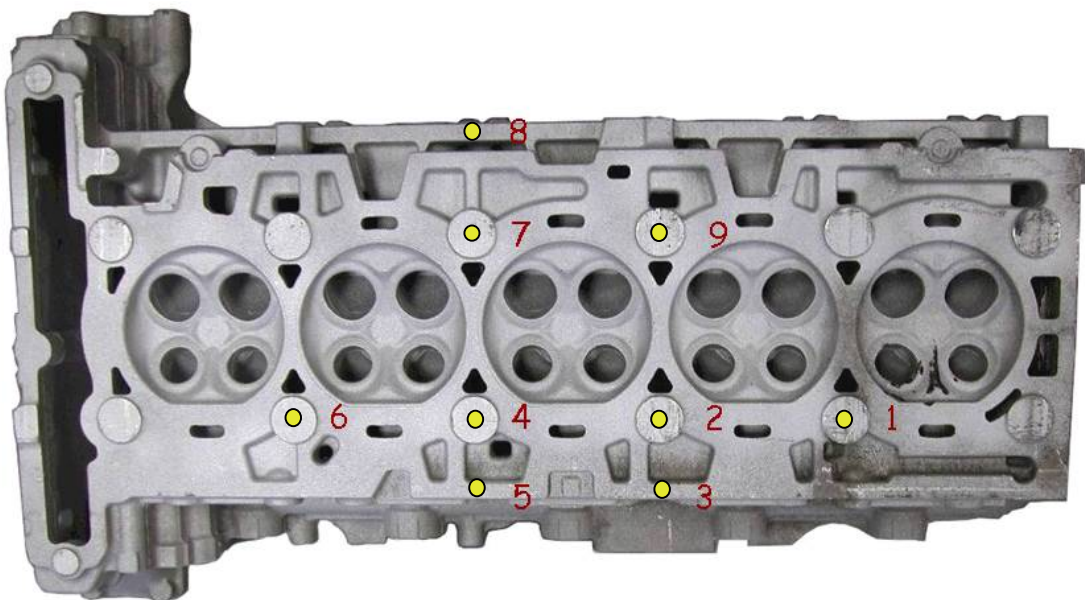
Figure 1.3-22. Cast aluminum A356 engine head instrumented with K-type thermocouples [22]
