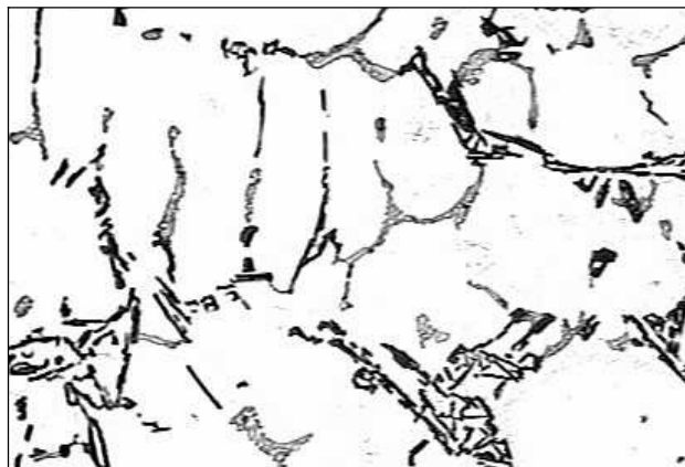
Figure 2.3-1. Al-6.5%Si-3.5%Cu, cast near a chill. White matrix is \alpha , dark gray particles are silicon, and light gray particles are \theta -phase. (Unetched, 350 X.)
