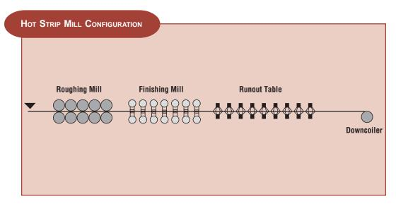
The Hot Strip Mill Model (HSMM) is a predictive tool that quanitatively links the properties of hot rolled product to the operating parameters of a conventional hot strip mill. The simulation model is complete and is being commercialized by INTEG Process Group, Inc.
