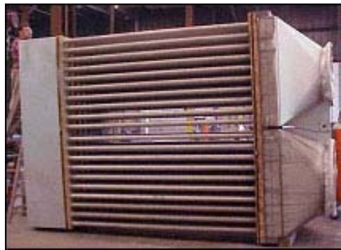
Figure 19. Typical recuperator used for steel reheating
