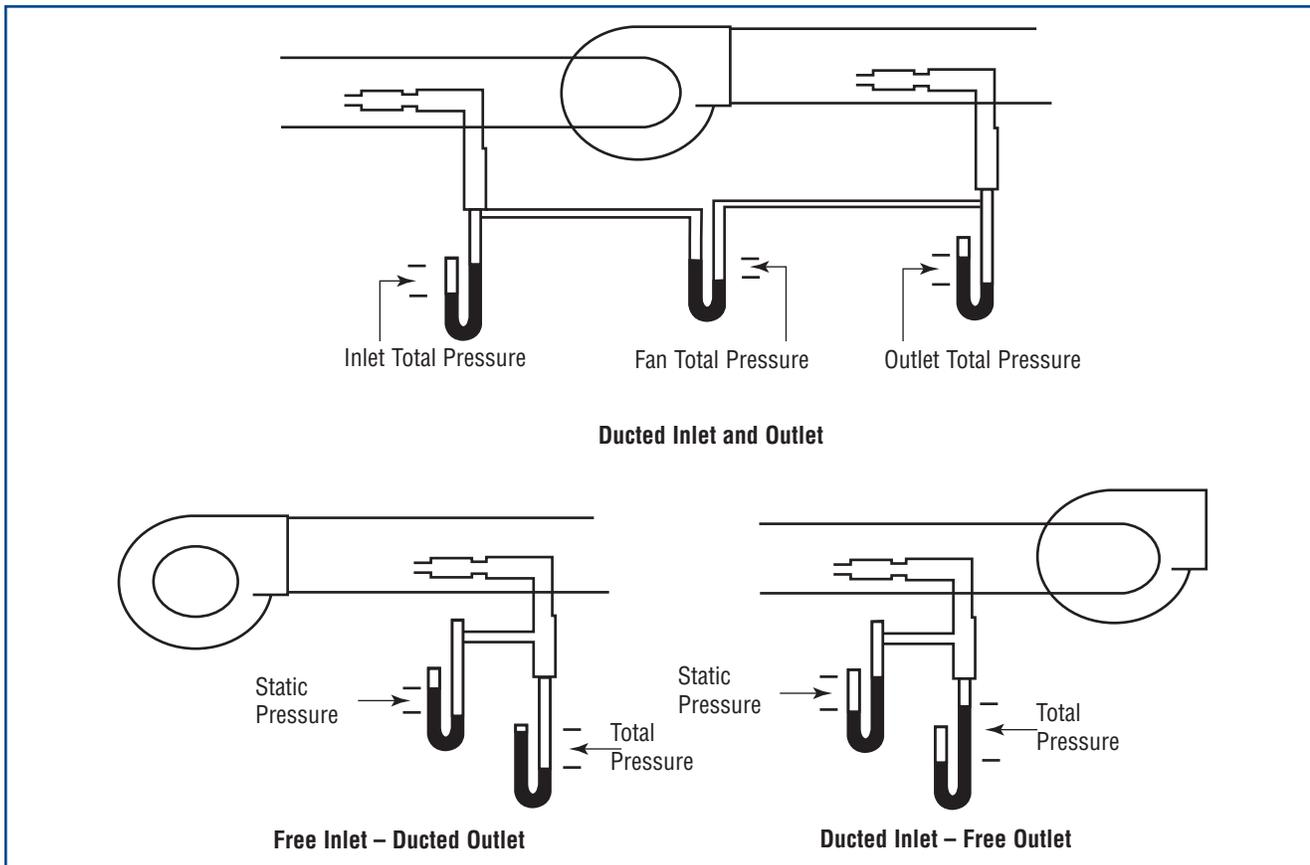
**Figure 2-28. Alternative Methods of Measuring Fan Pressure**
