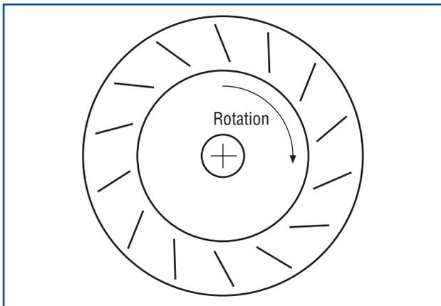
**Figure 2-6. Backward-Inclined Fan**
