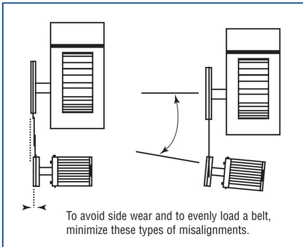
Figure 2-23. Improper Alignment
