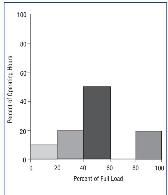
Figure 2-26. Load-Duty Cycle
