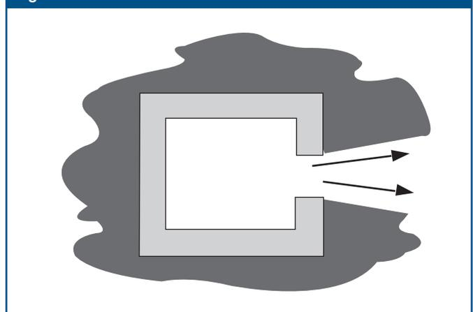
Anywhere or anytime there is an opening in the furnace enclosure, heat is lost by radiation, often at a rapid rate. These openings include the furnace flues and stacks themselves, as well as doors left partially open to accommodate oversized work in the furnace.
