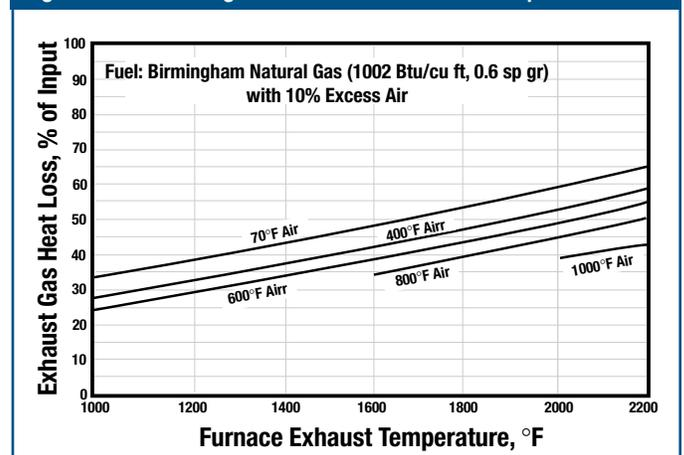
**Waste heat recovery.** Reducing exhaust losses should always be the first step in a well-planned energy conservation program. Once that goal has been met, consider the next level – waste heat recovery. Waste heat recovery elevates furnace efficiency to higher levels, because it extracts energy from the exhaust gases and recycles it to the process. Significant efficiency improvements can be made even on furnaces that operate
