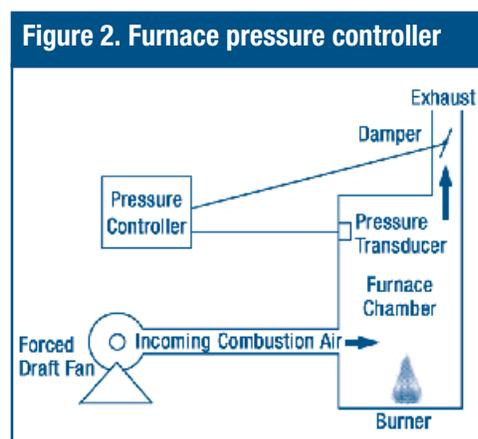
Pressure controllers can be manual or automatic. An equipment operator typically uses a dial on a control panel to set the pressure in a manual system. An automatic system has a feedback loop and continuously monitors and regulates the pressure through an electronic control system. A barometric damper is an inexpensive option for a natural draft furnace or oven.
