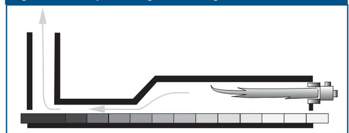
Figure 10. Exhaust gas losses with ambient and preheated air.
