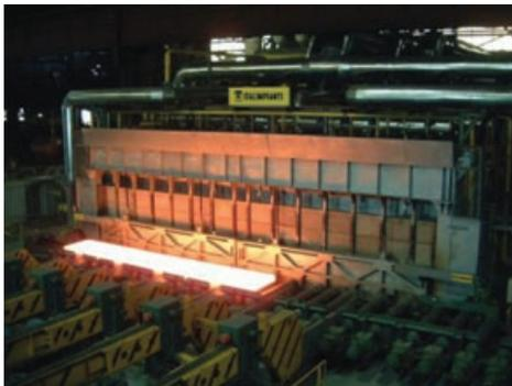
*A walking beam furnace for metal reheating.*
