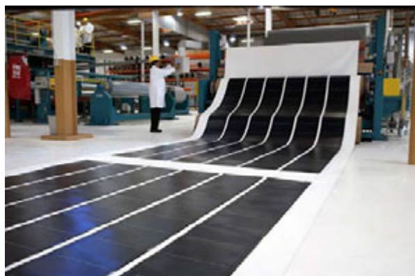
Fig. 2. The Uni-Solar a-Si factory produces peel-and-stick thin-film PV roofing material.
