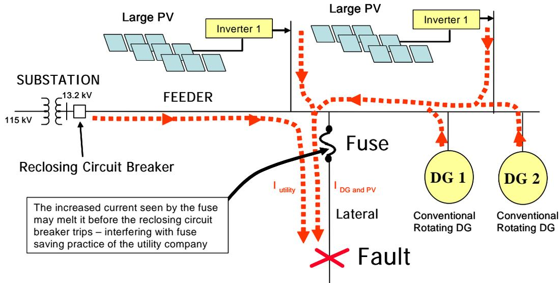
**Figure 2-9. How fault contributions from other feeder energy sources such as PV can interfere with fuse and circuit breaker coordination in fuse-saving schemes**
