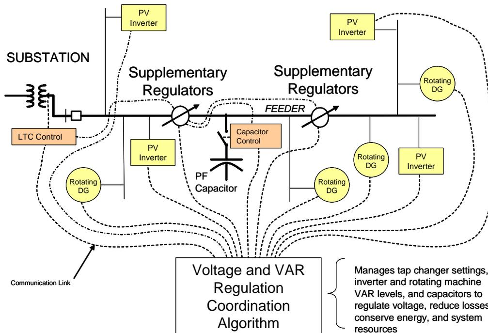
**Figure 3-2. Integrated voltage regulation scheme for utility feeders with high-penetration PV and other DG energy sources**
