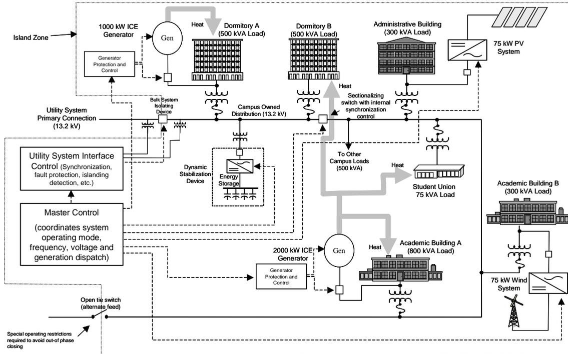
**Figure 3-9. Conventional radial campus distribution system converted to a microgrid**
