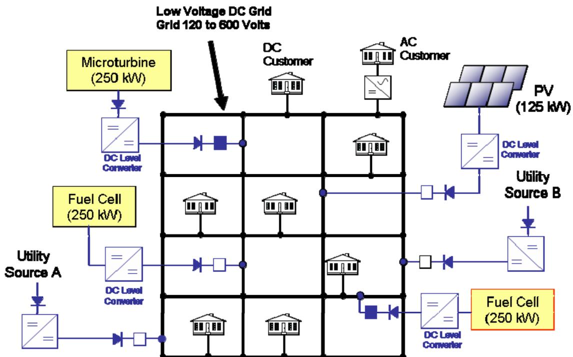
Figure 3-13. An LV DC grid network, rich in DG, for suburban and light urban areas (section current limiter omitted for clarity)
