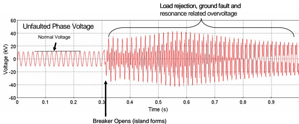
**Figure 2-13. Examples of simulation of ground fault overvoltage, load rejection, and resonance-related overvoltage**
