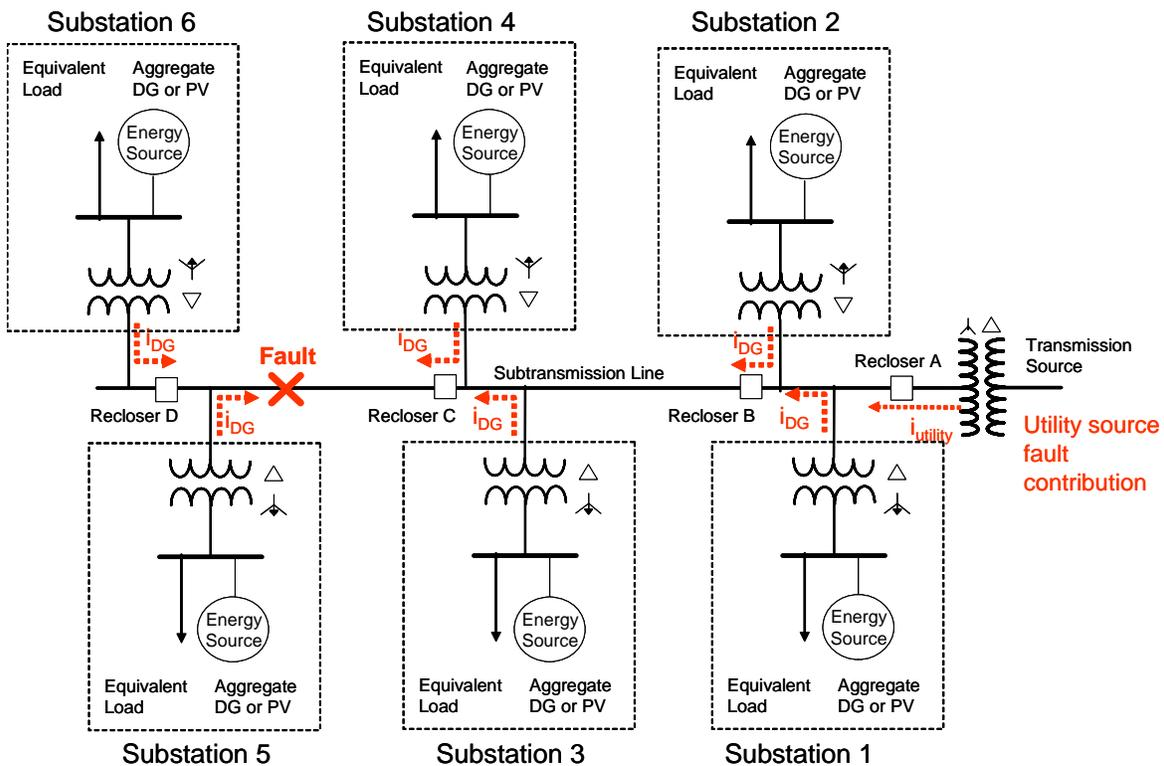
**Figure 2-15. Aggregation of distribution-connected PV and other DG resources at many distribution substations can have a significant impact on subtransmission fault levels, affect the switching schemes, pose an islanding risk, and cause ground fault overvoltages**
