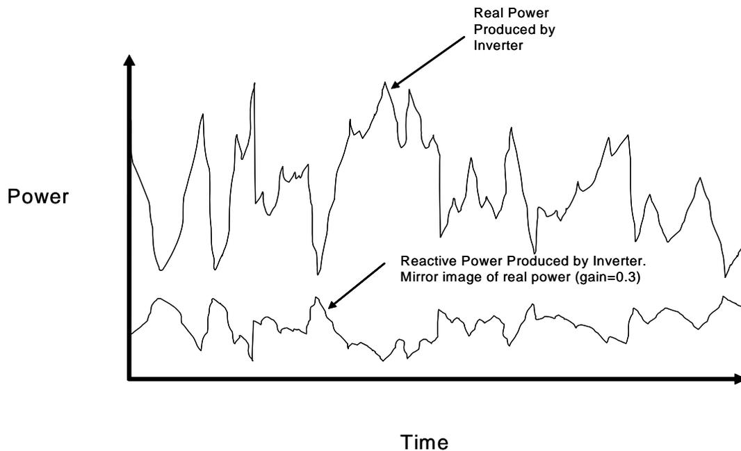
**Figure B-5. Inverter mirror image reactive power compensation to help reduce the voltage change effects resulting from PV power variations (could be an autonomous algorithm)**
