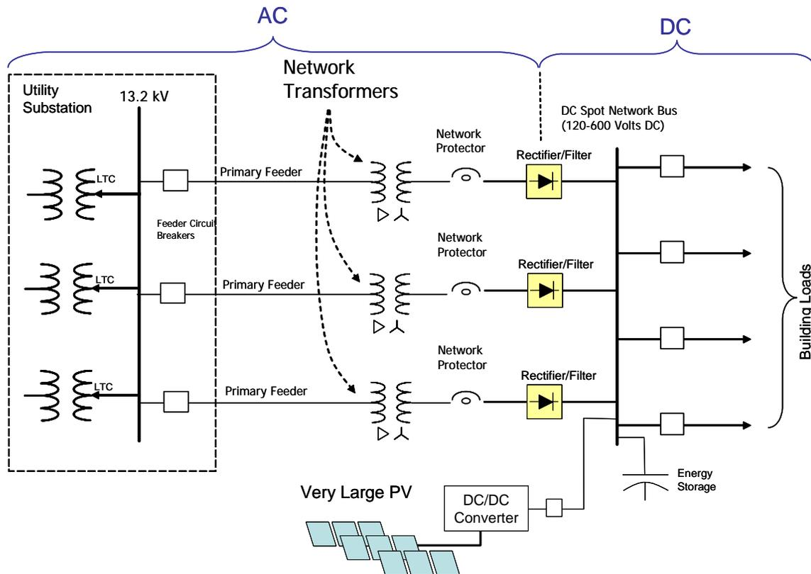
**Figure 3-12. An LV spot network partially converted to DC solves protection problems associated distributed energy sources located on LV networks**
