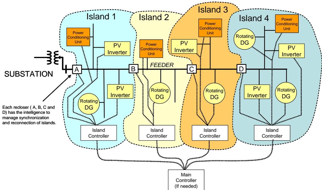
Figure 3-5. Four-island distribution feeder
