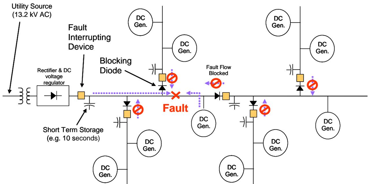
**Figure 3-10. Fault and voltage sag blocking concepts using DC distribution, diodes, and energy storage.** The DC generator sources can be PV or other types of distributed energy sources.
