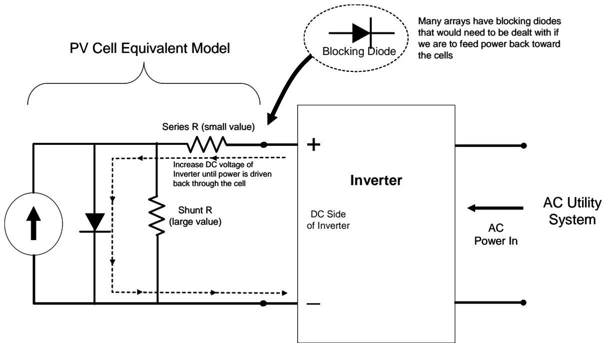
**Figure B-4. Using a solar array as an energy absorber to provide system damping and suppression of transient overvoltage conditions**
