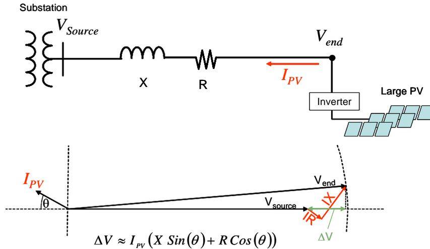
**Figure 2-3. Approximate voltage rise resulting from injected current of PV system**
