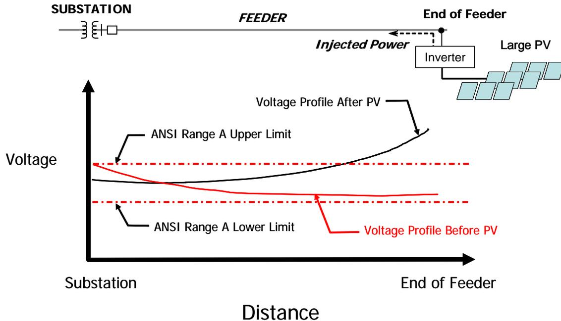
**Figure 2-4. Tail end of regulation zone forced to high voltage because of large exporting PV system located near the end of the feeder or regulation zone**
