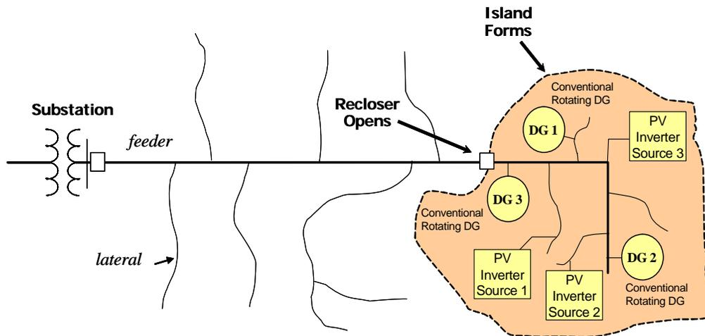
**Figure 2-10. Example of an island composed of conventional rotating machine energy sources and PV inverter sources**
