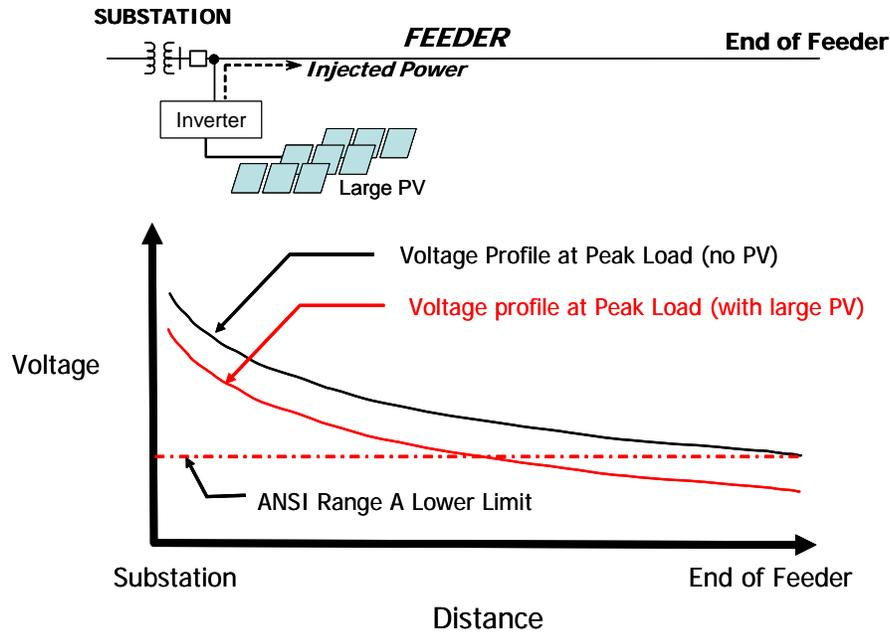
**Figure 2-2. Line drop compensation-controlled voltage regulator allows undervoltage at the end of the feeder when the PV generator injects power**
