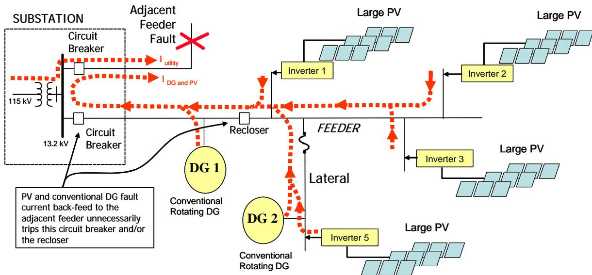
Figure 2-8. Example of how high penetration of DG can cause nuisance trips
