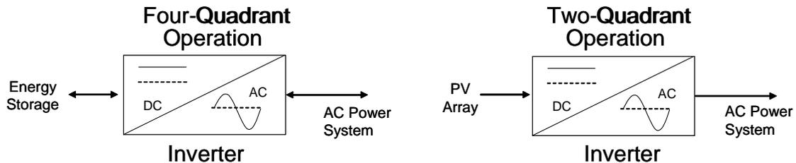
Figure B-2. Inverter devices capable of two- and four-quadrant operation
