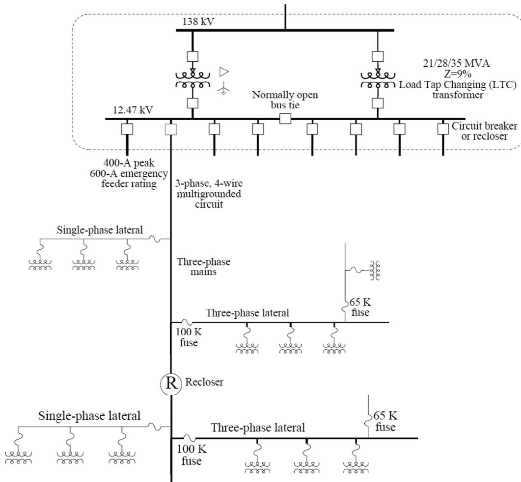
Figure 2-1. Typical distribution feeder topology [1]
