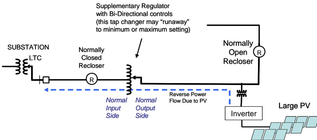
**Figure 2-5. Runaway tap changer on an autoloop supplementary regulator results from reverse power detection**
