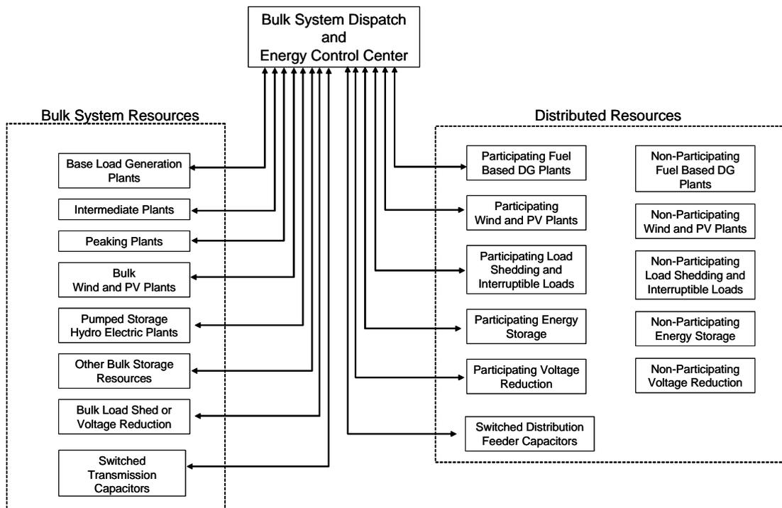
**Figure 3-3. Resources available to the independent system operator (ISO) and/or bulk system control center in the 21st-century power system (some resources can be fully dispatched and others are simply monitored or ramped down as needed)**
