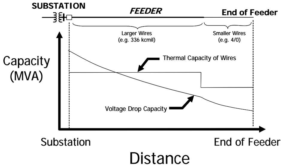
**Figure A-15. The capacity of a feeder changes as one moves further from the source.** Capacity is the lesser of either the voltage drop or thermal limits at the point of interest.
