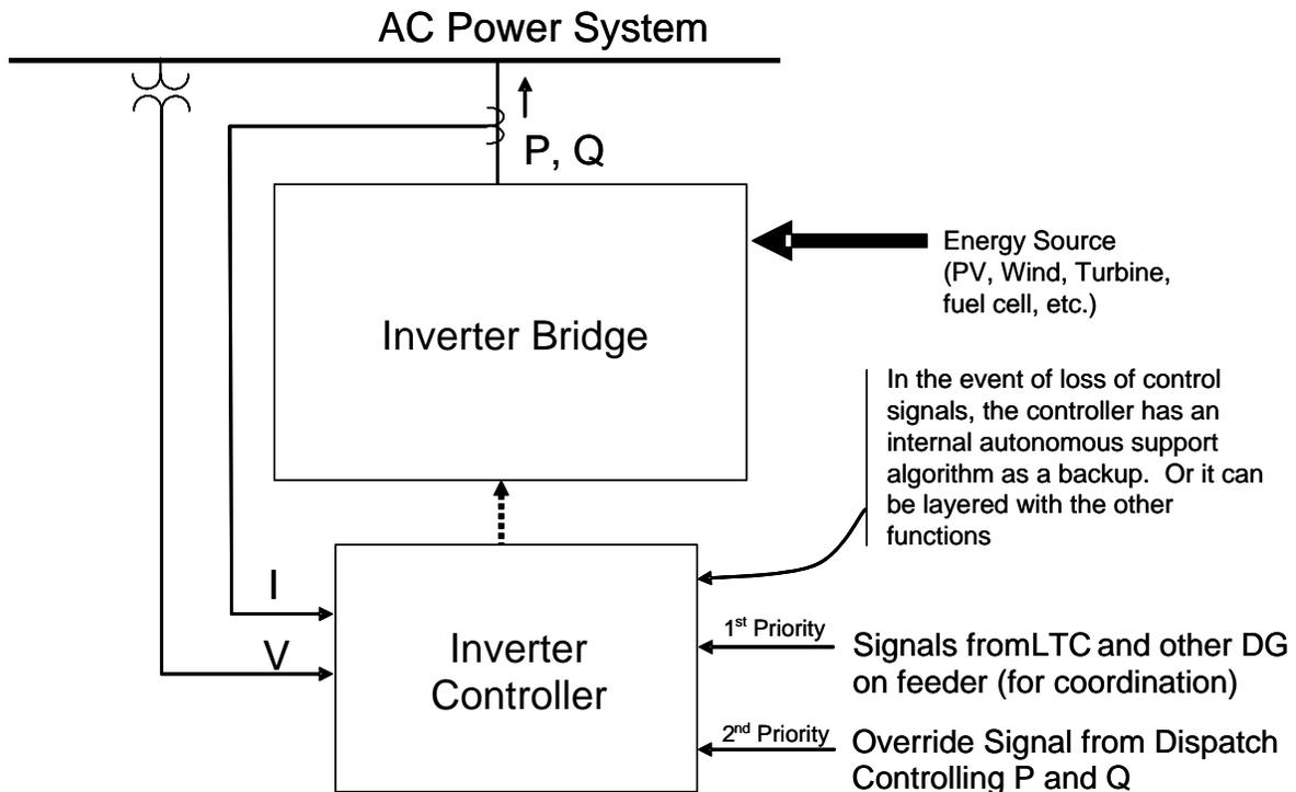
Figure B-3. Features of an inverter with active control capability
