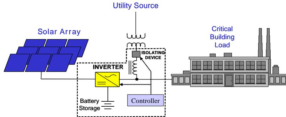
**Figure B-6. Functional arrangement of a PV device that can operate in parallel with the utility system but can instantly and seamlessly transition to microgrid mode to support a critical load**
