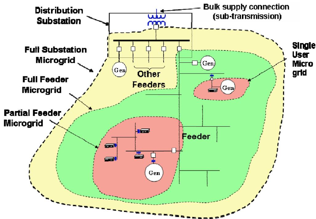
**Figure 3-8. Examples of microgrids on a radial distribution system—from a single customer up to an entire substation**
