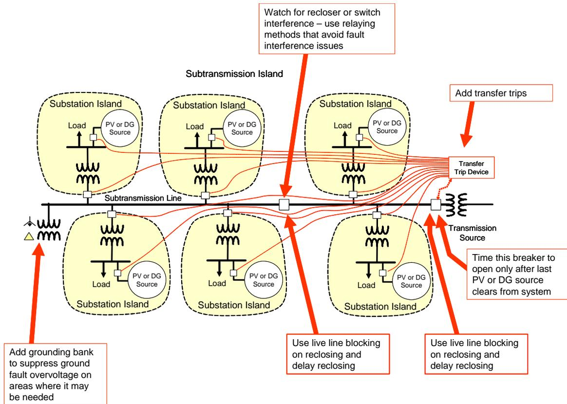
Figure 3-14. Subtransmission issues and upgrades to handle higher penetration of PV
