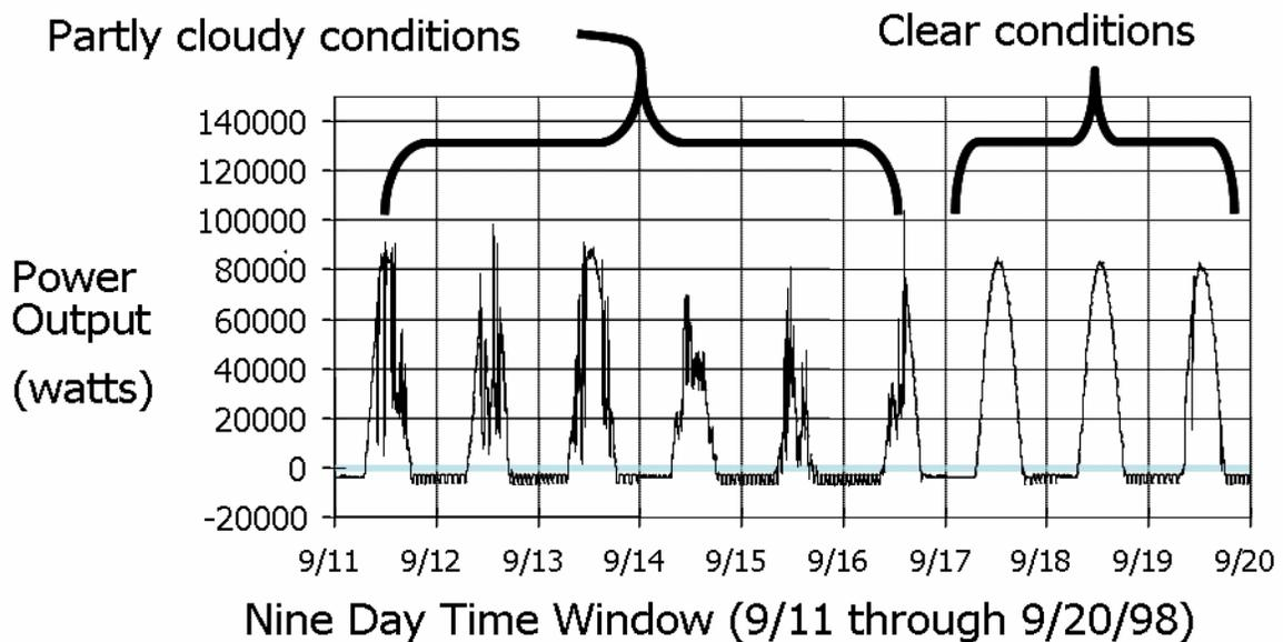
**Figure 2-6. PV power fluctuations at a 100-kW PV site near Albany, New York**
