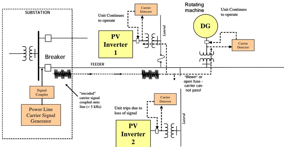
**Figure 3-4. Power-line, carrier-based, pilot-relaying scheme for anti-islanding protection**
