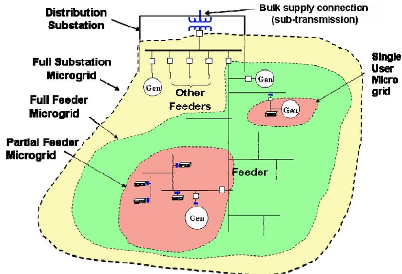
Figure ES-3. Concept of distribution microgrids of various sizes and levels, allowing reliability islands and grid tie operation
