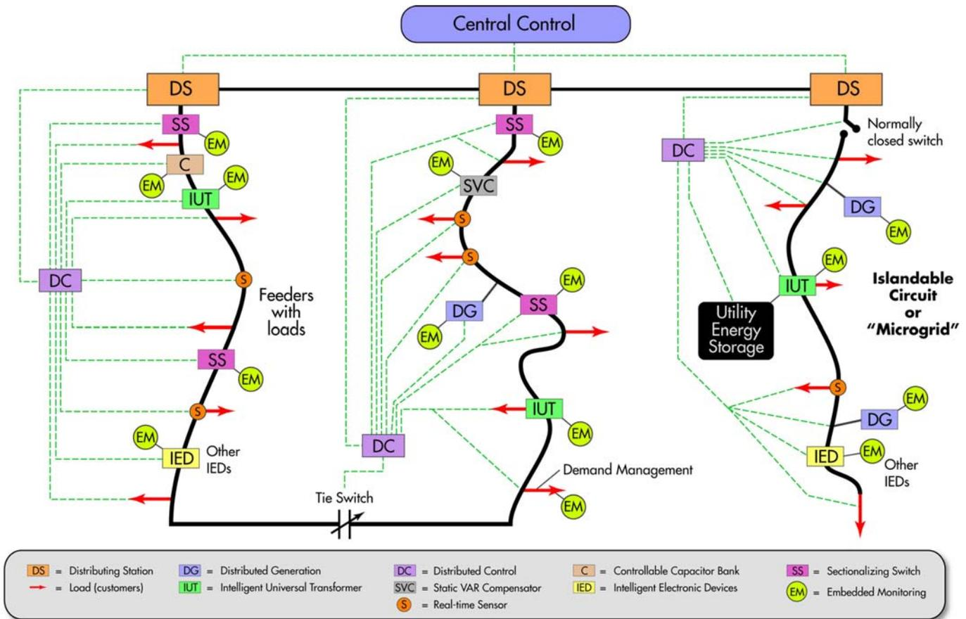
**Figure 3-1. Future devices in an advanced distribution system**
