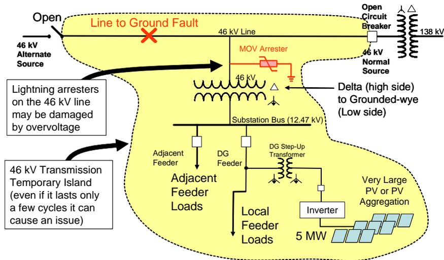
**Figure 2-14. Ground fault overvoltage that can occur on subtransmission in some high-penetration PV or DG scenarios**
