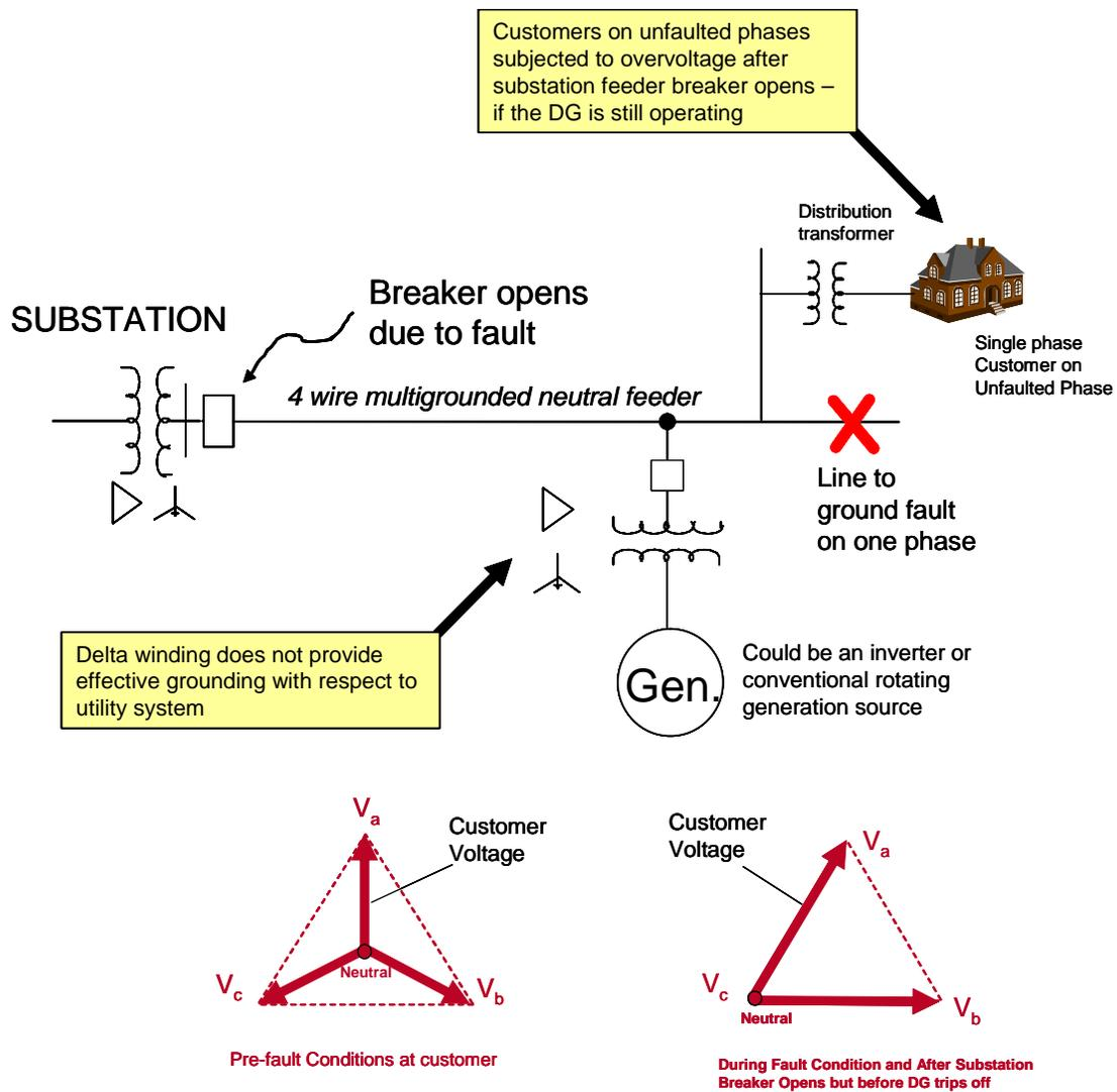
**Figure 2-12. Delta windings on the high side of distributed energy source interface transformers act as one possible form of an ungrounded source and can cause ground fault overvoltage damage**
