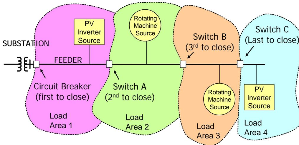
**Figure 3-6. Use of cascaded restoration switches to allow PV and other feeder energy resources to help with load pickup**
