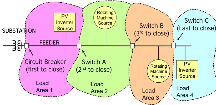
**Figure ES-2. Illustration of cascaded restoration of DG**
