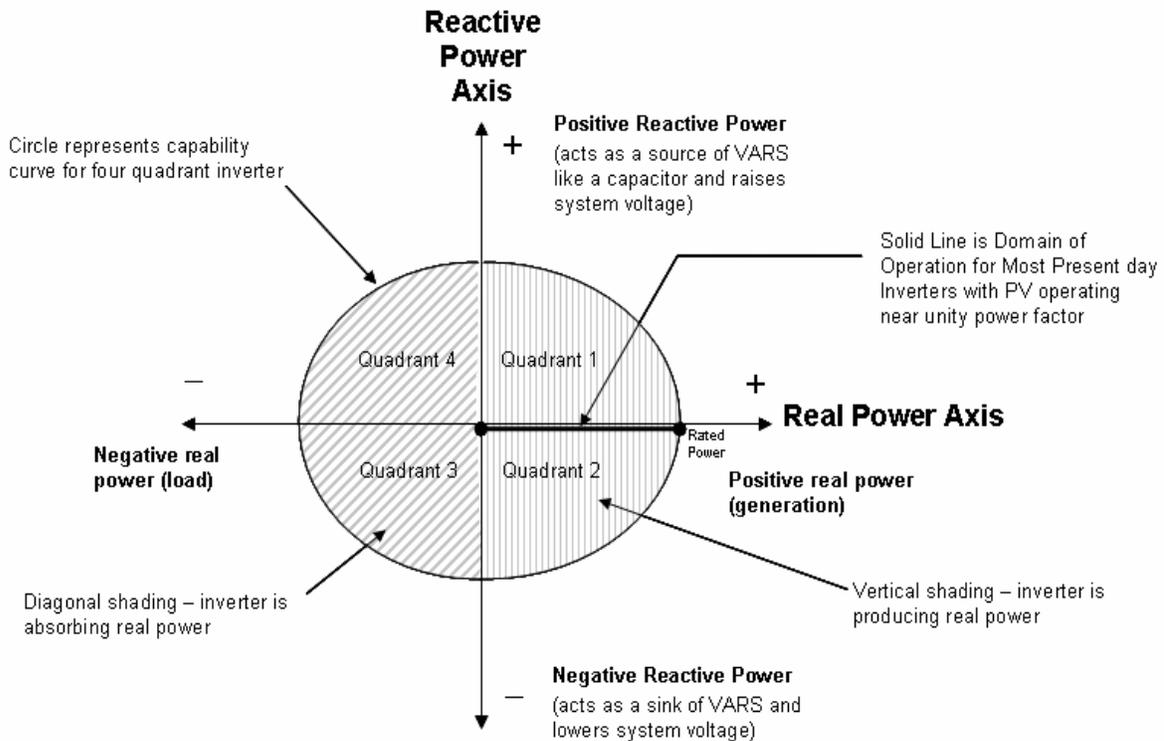
Figure B-1. Quadrants of inverter operation
