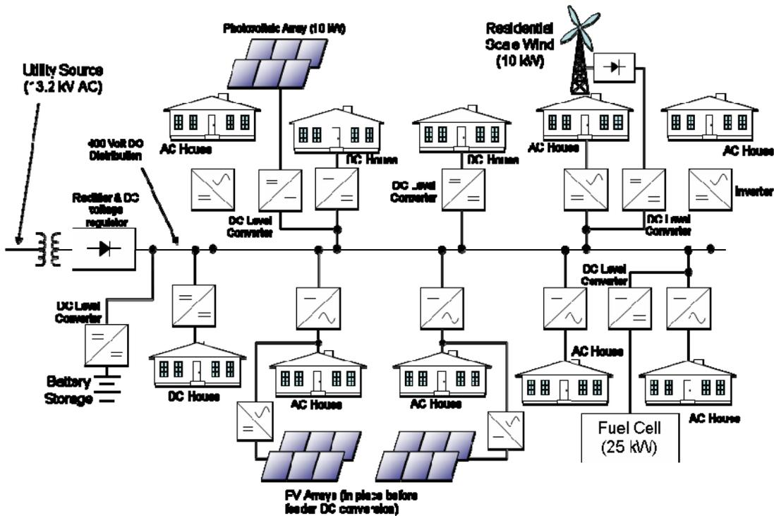
Figure 3-11. Residential single-phase lateral converted from 7620 V AC to 400 V DC with high-penetration DG
