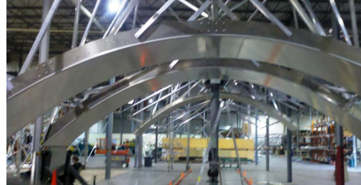
7m, 8m, and 9m mirror panels – contour measurements
