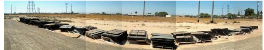
Photo 6: Panorama of poorly handled float glass a-Si for bid 2005.
