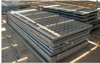
Photo 1: 2006 Stacked single crystal silicon salvage sales PV panels.
