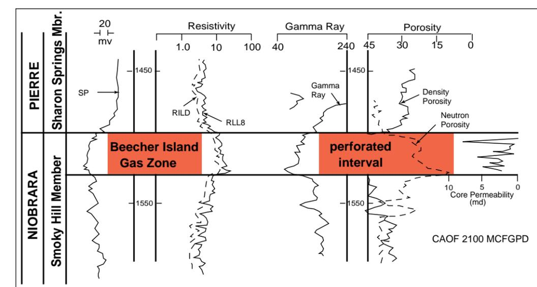
**Figure FB-16.6.** Type logs for Niobrara producing well, Beecher Island area, Kansas Nebraska No. 1-32 Whombie, sec. 32, T2S, R43W (after Lockridge and Sholle, 1978).
