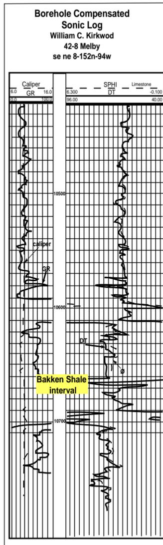
**Figure FB-15.3.** Example of log signature from Antelope Field showing Bakken shale interval with sand/silt development
