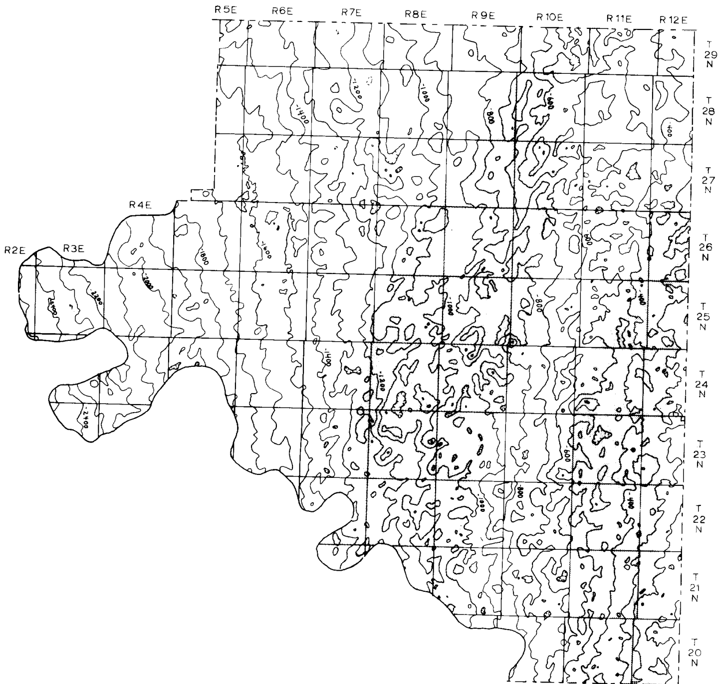
Figure 12. Structure contour map on top of Oswego lime in the Osage Indian Reservation. Contour interval 100 feet. Shaded zones show north-northeast-trending fold belts (from Bass, 1942).
