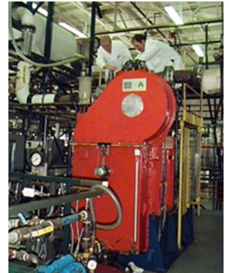
Figures. (Top) Wabtec single cylinder research engine (bottom) Progress Rail 4-stroke 16L 1010- single cylinder engine
