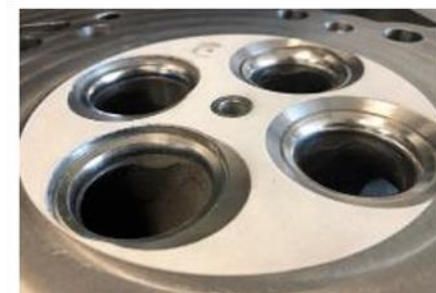
GdZr coating on cylinder head (example shown here)
