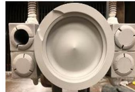
'Gen 3' coating on piston (example shown here)
