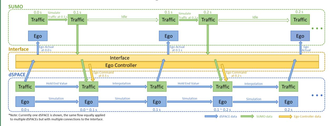
Traffic simulation SUMO normally runs much faster than dSPACE simulation. An ego controller sends speed command to dSPACE. The controller currently lives inside the Interface, but it can also live inside the dSPACE. dSPACE simulates the actual speed of ego vehicles and sent to SUMO.
