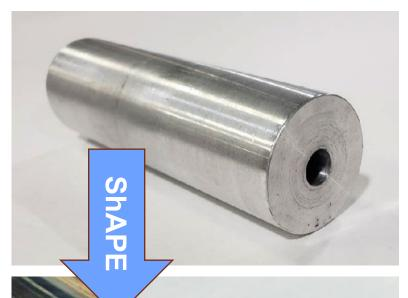
12 mm OD2 mm wall4.2 meters/min
