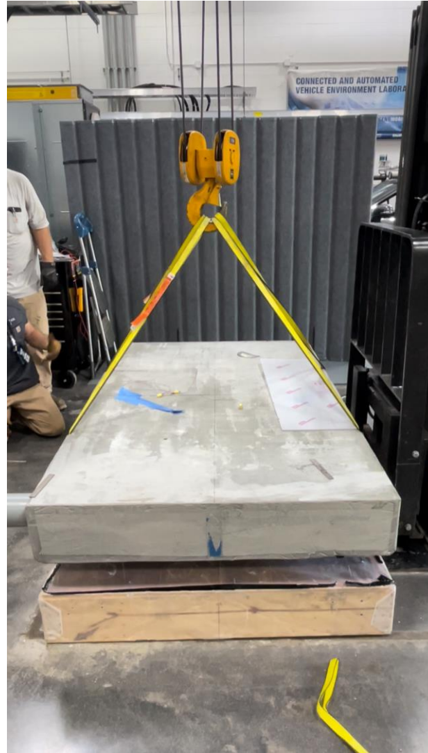
200 kW DWPT system with transmitter set in precast Master flow 648 Epoxy Resin Grout
