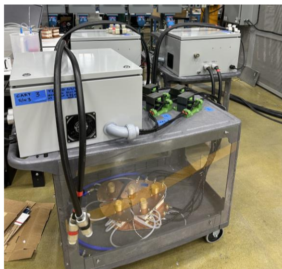
4 primary side HF power electronics units
