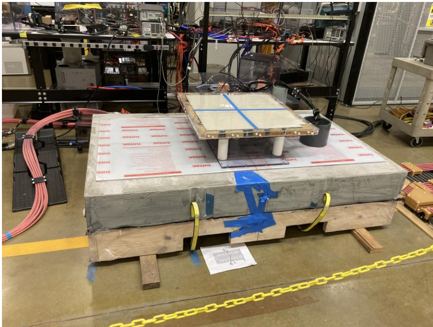
200 kW DWPT system with transmitter set in precast Master flow 648 Epoxy Resin Grout
