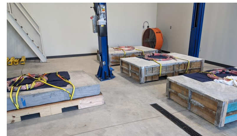
Coils with fiber glass re-enforcement being concretized
