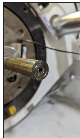
Image (left) and schematics of square wire extrusion tooling designed for ShAPE of composite magnet wires
