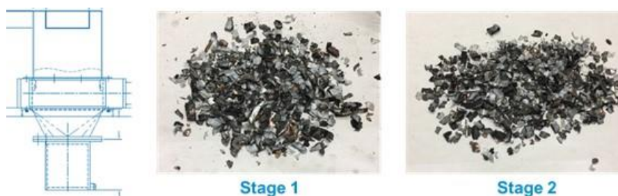
Figure I.3.C.39 Single-stage and two-stage shredding of pristine pouch cells in a submersible shredder
