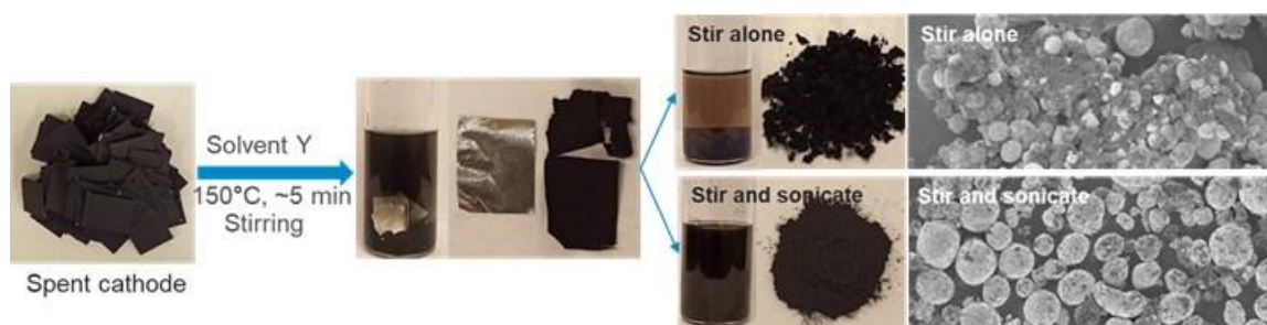
Figure I.3.C.42 Diagram with photos showing the recovery of spent cathode in the solvent Y (left) and digital images and SEM images showing the differences between stir alone and stir & sonication (right).
