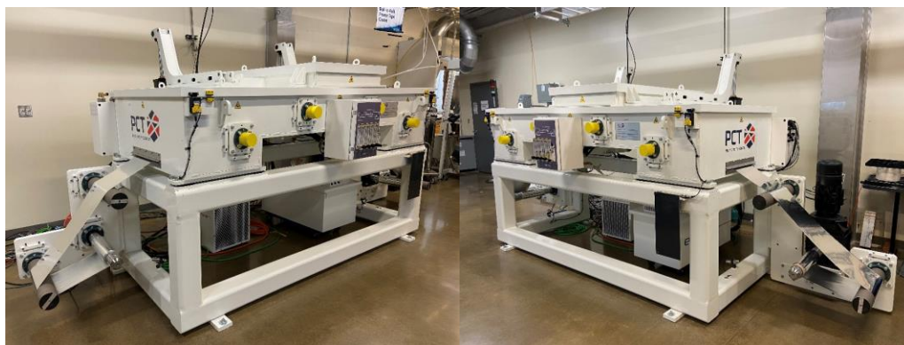
Figure I.2.A.3 The EB pilot line installed at Battery Manufacturing R&D Facility at ORNL (BMF).
