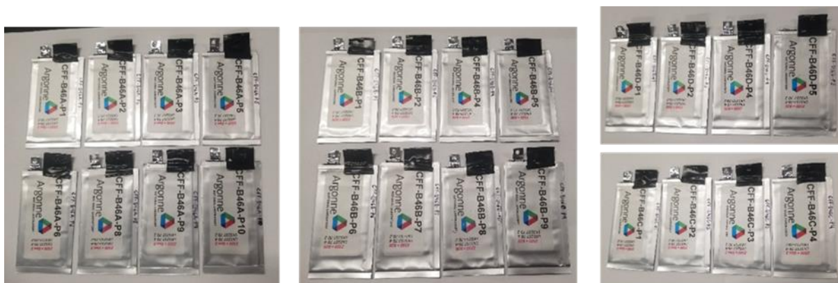
Figure I.4.M.28 Photo of fabricated pouch cells using low carbon and binder electrodes and selected electrolytes and separators for FY 2020 Milestone.
