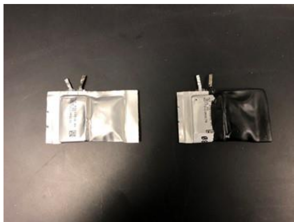
Figure II.3.G.9 Representative 200 mAh pouch cell following calendar life test (left). The top rubberized coating layer is visible post-calendar life test (right)
