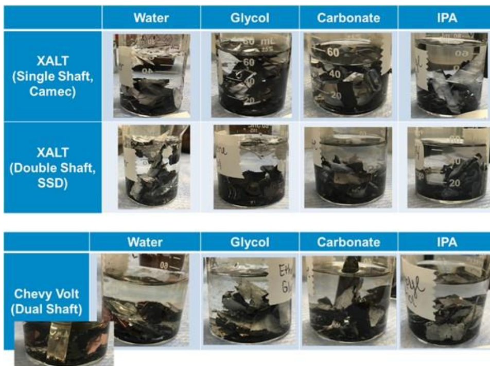
Figure I.3.C.49 Flotation experiments using water, glycol, carbonate, and isopropyl alcohol (IPA) on shredded pristine pouch cells (top) and end-of-life cells (bottom)
