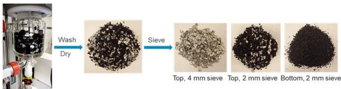
Figure I.3.C.41 Diagram with photos showing the delamination in a CSTR and separation of cathode films from Al foils through sieving.
