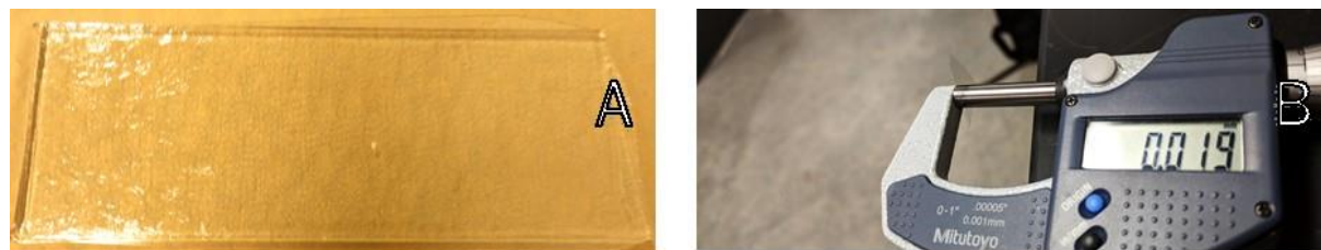
Figure II.9.F.6 (A) Full size preform (10cm x 30cm x 1cm) of LiPO3 glass (B) Drawn thin-film ribbon of LiPO3 glass thin-film (19 \mu\text{m} ).
