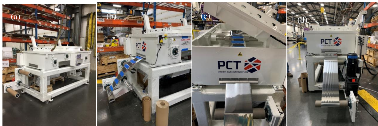
Figure I.2.A.1 (a) overview of the framework of the EB pilot line. (b) the unwind front, (c) web passing through the chamber, and (d) the rewind end of the pilot line during the factory acceptance.
