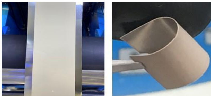
Figure II.9.E.1 (left) a separator film coated by a slot-die coater; (right) flexibility of the separator
