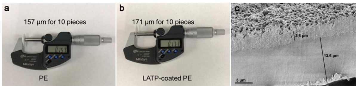
Figure II.13.A.27 Photograph of the recorded thickness of (a) PE and (b) LATP-coated PE separator by a micro-meter caliper. (c) SEM image of the cross-section of the LATP-coated PE separator.
