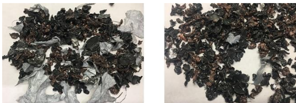
Figure I.3.C.36 Detailed images of sieved fraction >5.6 mm after hammermilling showing size difference of separator vs. foil (left) and abrasion of graphite film from copper current collector (right)
