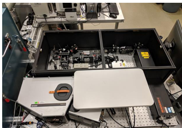
Figure I.2.D.2 Custom Raman spectrometer with in-situ sampling
