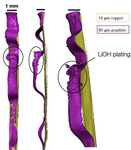
Figure I.4.K.35 3D visualizations of the cycled graphite anode showing copper current collector and thickness of LiOH plating on graphite anodes.
