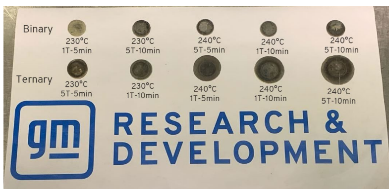
Figure XVI.10.3 Pictures of binary and ternary glass samples after hot pressing trials. All samples contained 3 wt.% bulk Kevlar fiber to improve strength and handleability.
