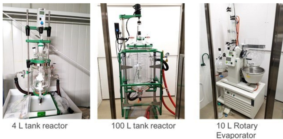
Figure III.3.76 Equipment that can be used to scale up the rinsing and concentration processes to recover spent electrolyte.
