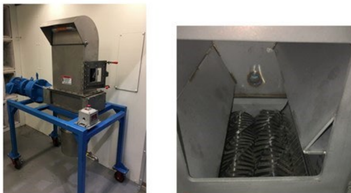
Figure III.3.58 ReCell's pilot-scale, submersible dual-shaft shredder
