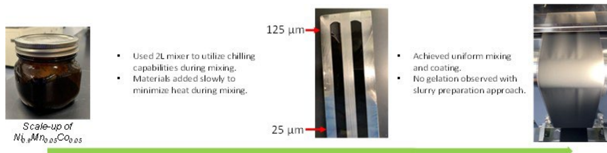
Figure VI.5.5 Scaled-up batch (200 grams) of \text{Ni}_{0.9}\text{Mn}_{0.05}\text{Co}_{0.05} provided to the CAMP Facility to produce >1.5 Ah pouch cells. Mixing sequence and control of temperature aided in creating a well dispersed slurry dispersion and uniform electrode.
