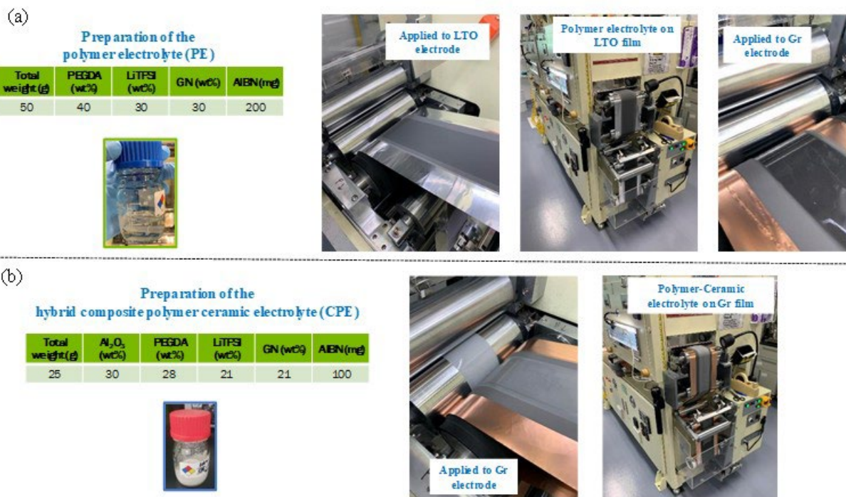
Figure VI.5.1 Images of the (a) polymer electrolyte [PE] coatings on LTO and graphite electrodes and (b) hybrid composite polymer ceramic electrolyte [CPE] coatings on graphite electrodes. The PE and CPE successfully applied to the electrode via reverse comma and the polymerization was initiated during coating process heat-treatment.
