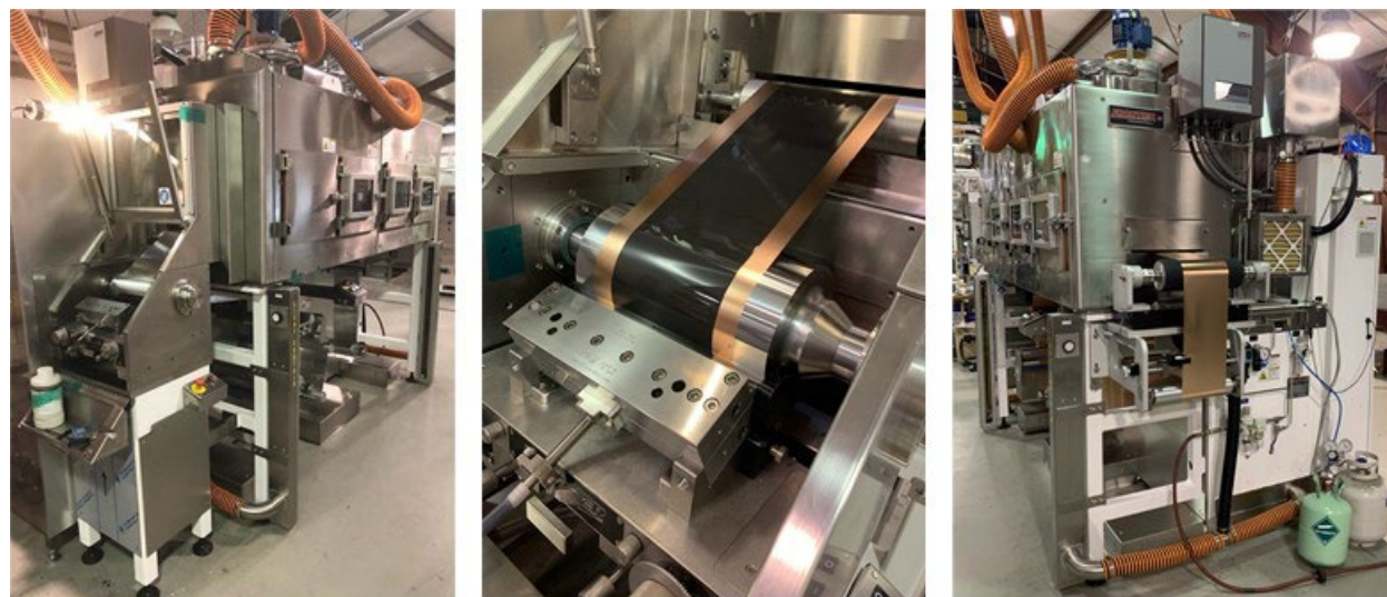
Figure VI.5.3 Images of the multifunctional coater during the FAT. The images are of the front end of the coater (left), slot die coating a CAMP Facility-made graphite anode slurry on copper foil (center), and back end of the coater (right).
