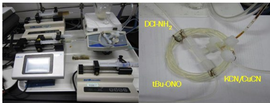
Figure II.4.10 Flow chemistry equipment and expanded view of coil reactor for Li-TCl
