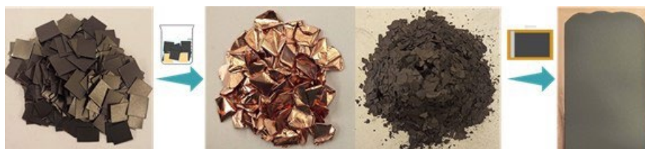
Figure III.3.60 Photos showing the direct recycling and remanufacturing of anode scraps using the newly invented SolveZ process.
