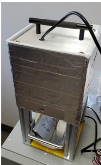
Figure III.3.90 Miniature nail penetration tester for low-temperature tests.
