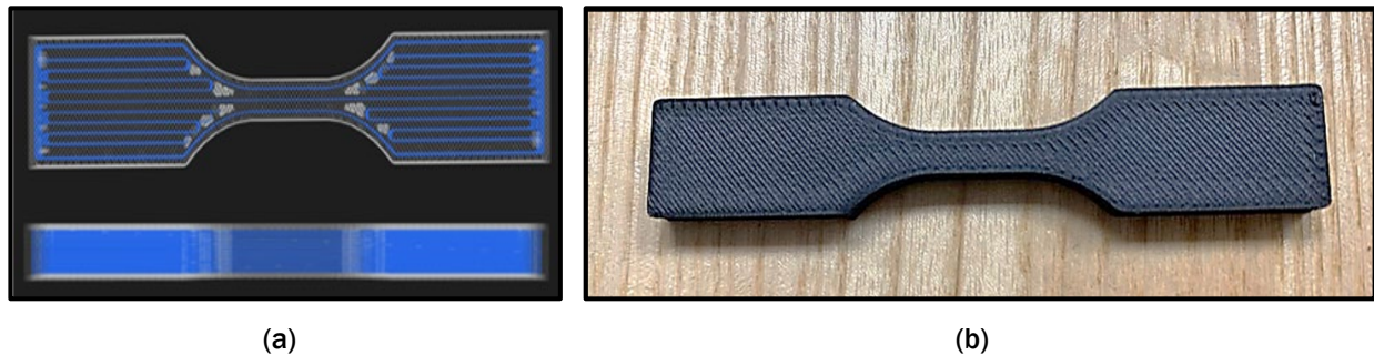
Figure II.2.20.2. (a) 2D rendering of the top and side build path and slicing diagrams of dog bones and (b) CCF 3D-printed dog bone. Source: SRNL
