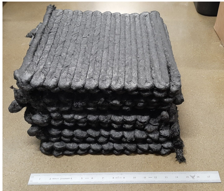
Figure II.2.11.9. AM preform made of long carbon fiber-reinforced PA66 (356-mm x 356-mm). Source: ORNL.
