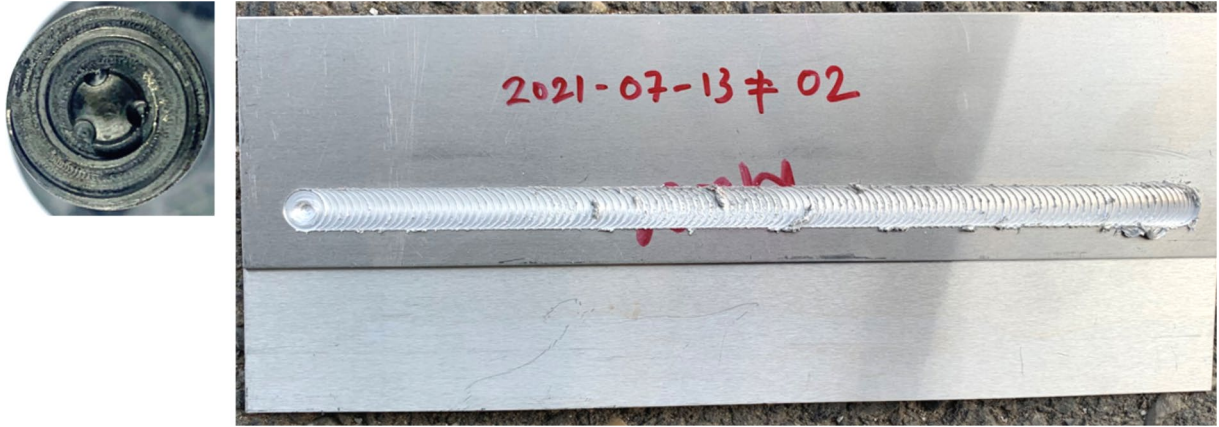
Figure II.3.2.1. FSW tool used to weld Al and Mg sheet and the Al side of the linear FSW Al-Mg welded panel. Source: PNNL.
