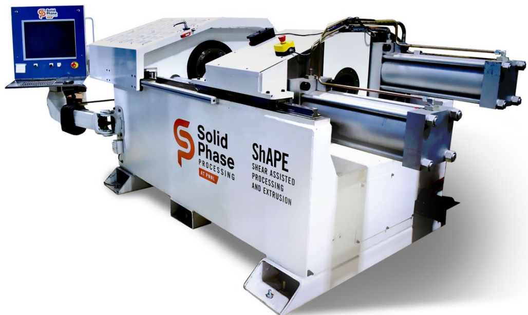
Figure II.1.1.1. ShAPE™ machine installed in PNNL's Solid-Phase Processing Laboratory. Source: PNNL.
