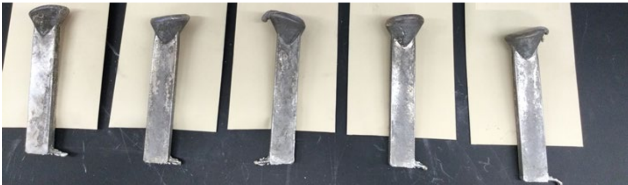
Figure II.1.5.5. Photograph of several candidate alloys used for screening. Source: ORNL.
