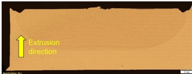
Figure II.1.11.6. (a) Example of Al-MMC rod made by ShAPE process. (b) An optical observation of the remnant puck. (c) The extruded rod along the longitudinal direction. Source: PNNL.
