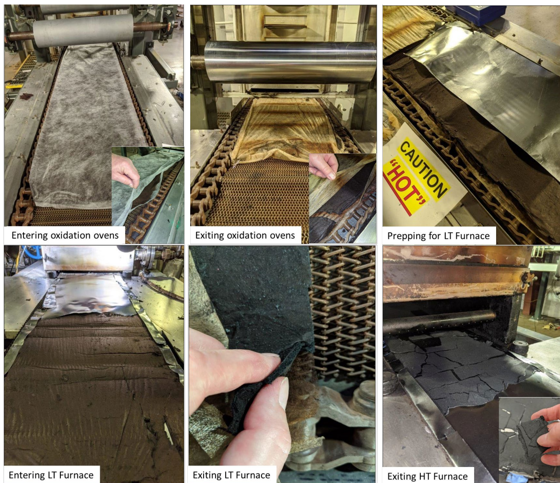
Figure II.2.7.4. Pitch-based precursor processed through the CFTF CF line. Source: ORNL.
