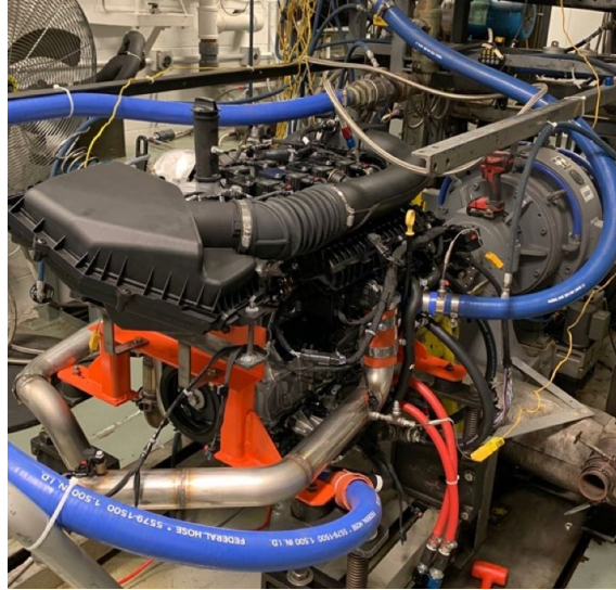
Figure I.1.2.4. The GM 2.0L turbo platform being utilized for component-level validation mounted to a dynamometer in Cell 14 at the Plymouth Technical Center. Source: Tenneco, Inc.
