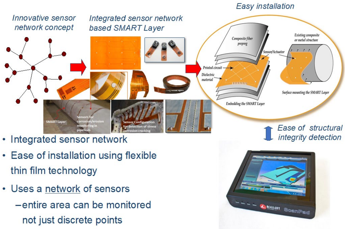
Figure II.4.2.1. SMART Layer sensors. Source: Acellent.
