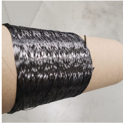
Figure II.2.7.10. CF produced with the OPF at CFTF. Source: ORNL.
