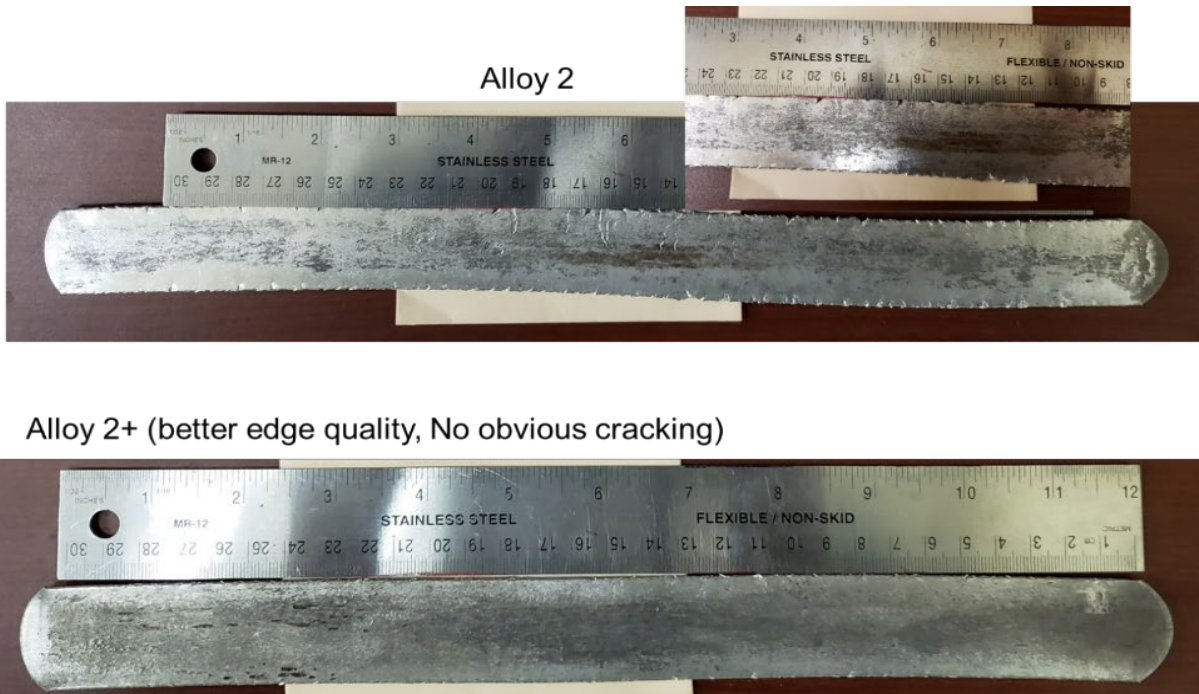
Figure II.1.2.5. Alloy 2 and Alloy 2 Plus sheets rolled to large reductions at 275 °C. Source: The Ohio State University.
