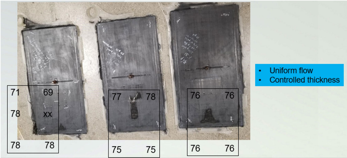
Figure II.2.13.11. Process repeatability and dimensional checks for a 200 g injected at 50 g/sec. Source: Michigan State University.
