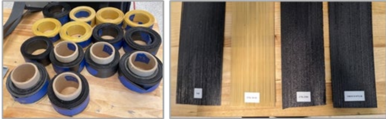
Figure II.2.12.14. Thermoplastic prepreg tapes produced for continuous tow development. Source: Ford.
