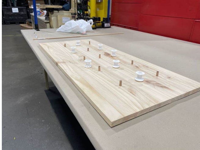
Figure II.2.12.20. Fixture to conduct preliminary end-effector capability studies. Source: Yanfeng.
