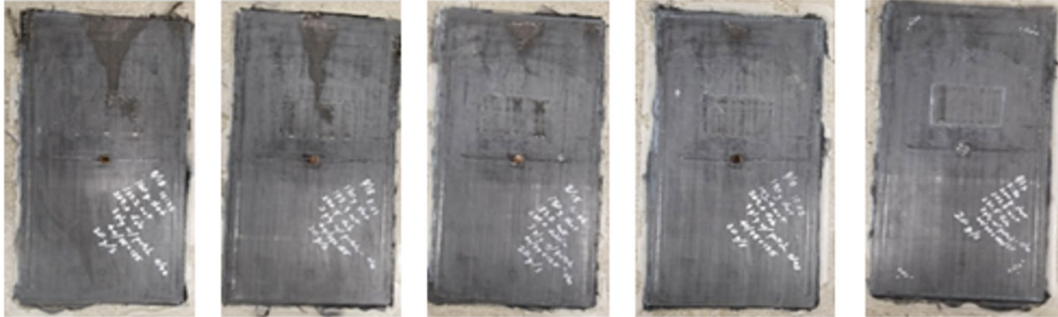
Figure II.2.13.10. Flow front progression for molded panels with different amounts of injected resin. Source: Michigan State University.
