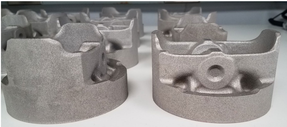
Figure I.4.2.16. Additively manufactured pistons with an AlCeNiMnZr alloy. Source: ORNL.
