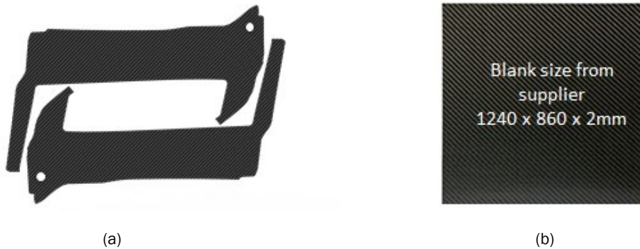
Figure II.2.3.11. (a) Inner beltline stiffener blank strategy; and (b) the blank size (1240 × 860) obtained from the supplier. Source: Clemson University.
