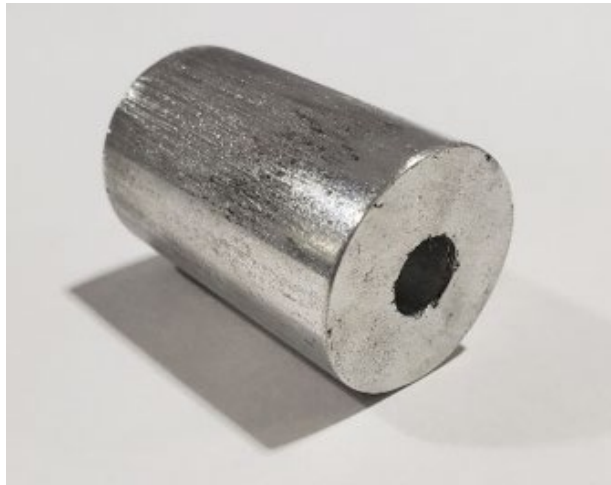
Figure II.1.1.4. Briquette manufactured by Magna R&D from 6063 scrap. Source: Magna R&D.
