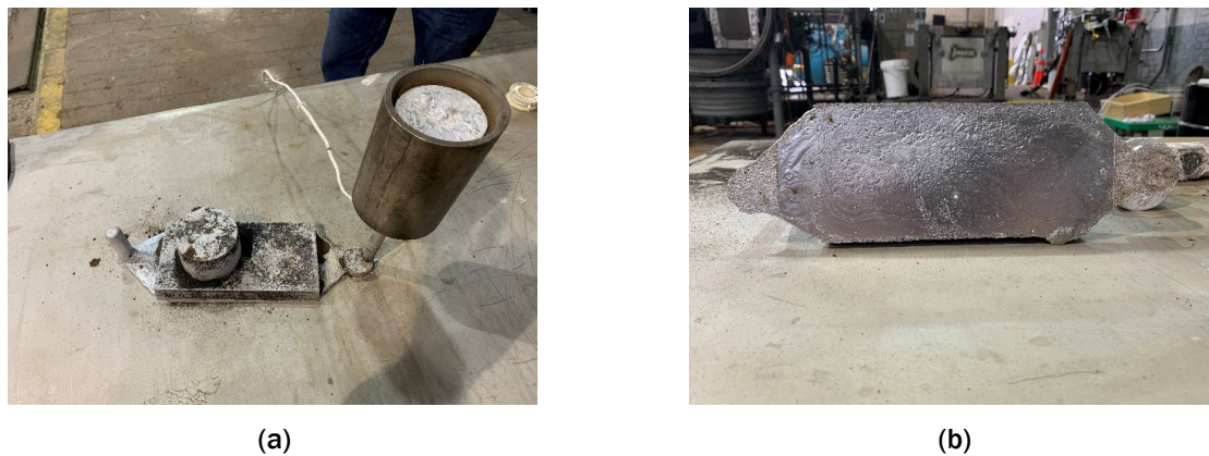
Figure II.1.3.7. A more recent Al plate (21-A35) cast against the water-cooled chill. Note the restricted in-gate to minimize aspiration and addition of a successful riser (a). The surface in contact with the chill (b) exhibited what appeared to be flow lines which can be attributed to the liquid flowing across the chill and freezing in place sequentially. The cylinder head should not exhibit this since the liquid will flow up the chill rather than across it. Source: NETL.
