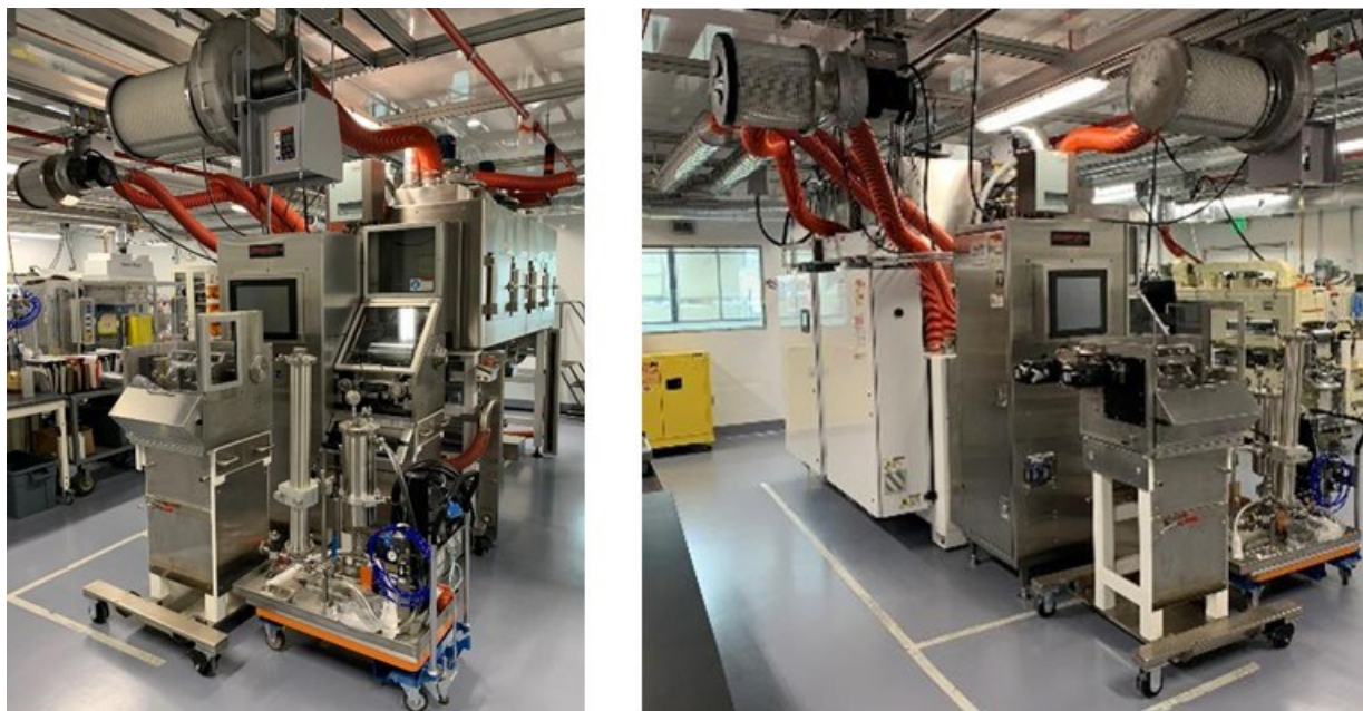
Figure V.5.1 Images of the multifunctional coater installed in the CAMP Facility's dry room.
