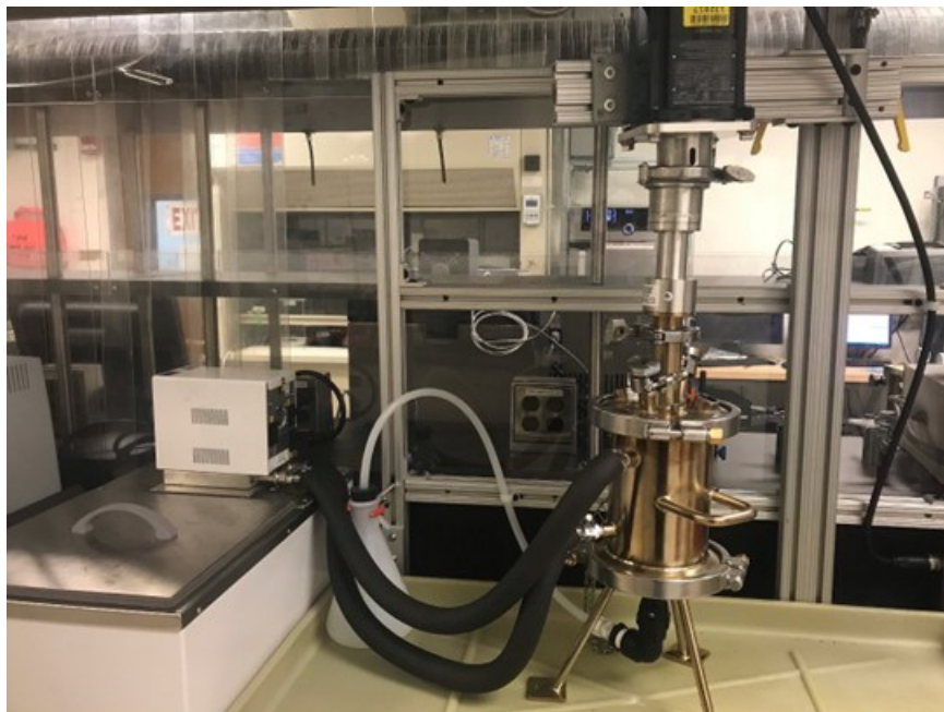
Figure III.3.19 Completed installation of 1L black mass purification reactor (Nutsche filter-dryer).
