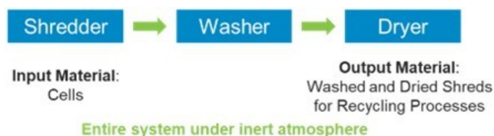
Figure III.3.2 Pilot-scale system designed and purchased for ReCell
