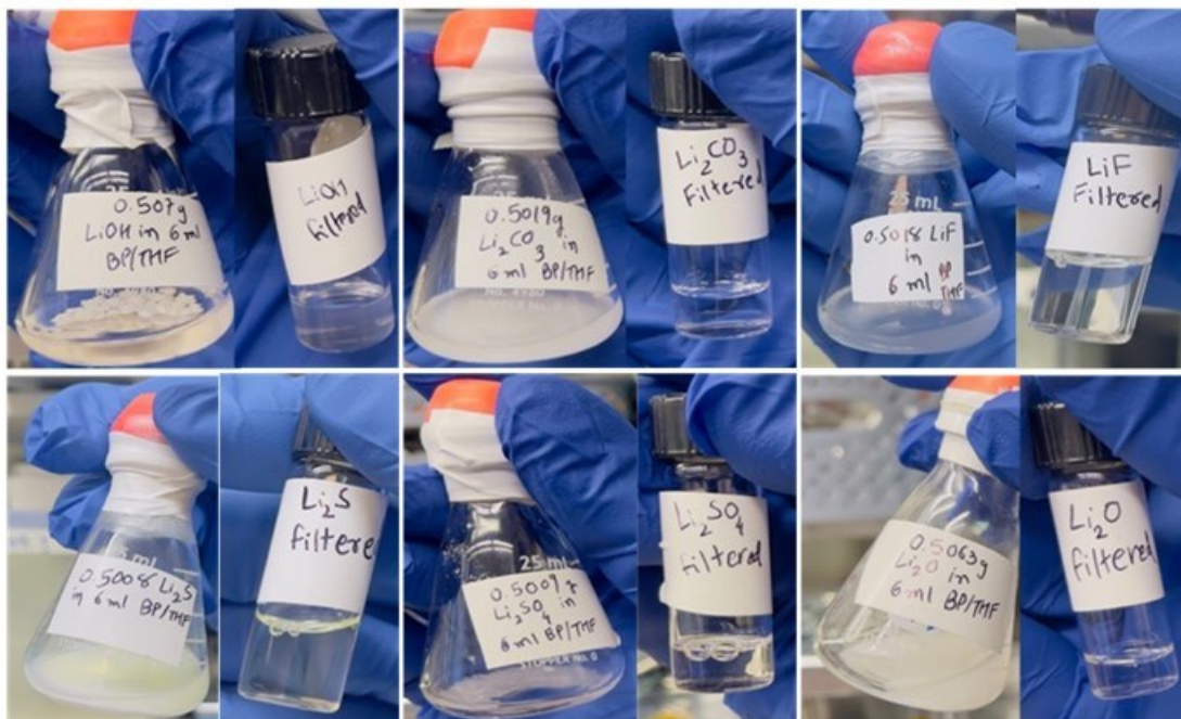
Figure XVII.1.106 Potential Li-S Batteries' SEI components (a) LiOH (b) \text{Li}_2\text{CO}_3 (c) LiF (d) \text{Li}_2\text{S} (e) \text{Li}_2\text{SO}_4 (f) \text{Li}_2\text{O} . before filtering (left) and after filtering (right)
