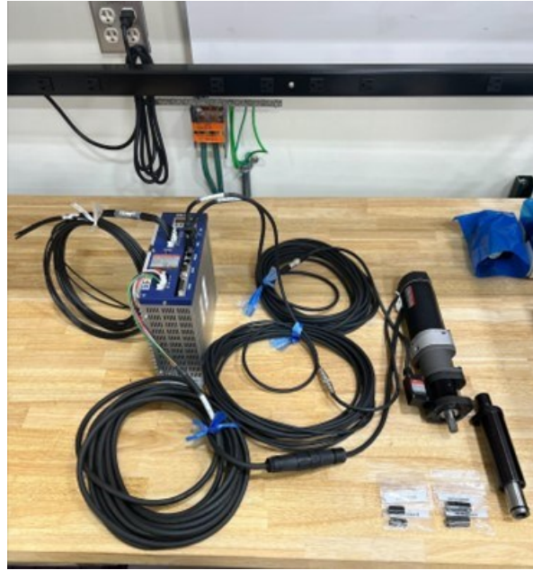
Figure III.3.55 (Estic custom ordered 80Nm high speed nutrunner with axial compensation connected on benchtop prior to robotic integration/Jonathan Harter)
