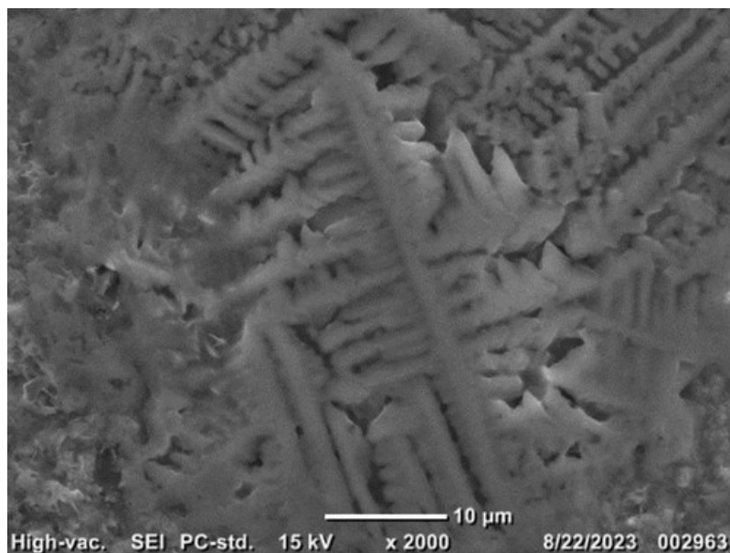
Figure XIII.25.7 SEM image of an electrolyte film after thermal annealing at 250°C.
