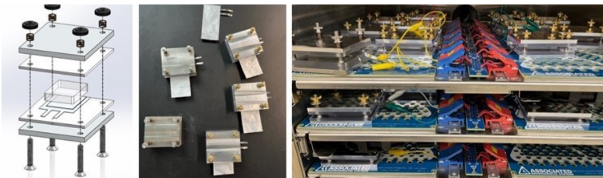
Figure VII.1.1 Single layer pouch cell fixtures and a temperature-controlled chamber enables calendar aging studies for various Si materials under controlled conditions.
