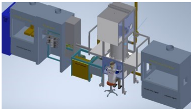
Figure II.2.4 FSP configuration for 500 g/hour production.
