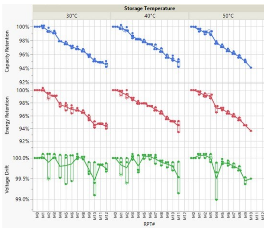
Figure I.10.3 C/3 capacity, energy, and nominal voltage retention during calendar life test for baseline cell chemistry.
