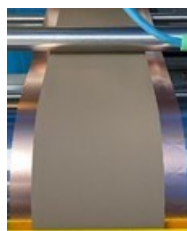
Figure VII.6.1 Continuous Si anode coating
