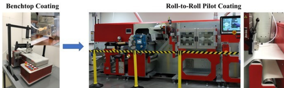
Figure II.13.1 Transition from benchtop coating to roll-to-roll pilot-scale coating at ANL.
