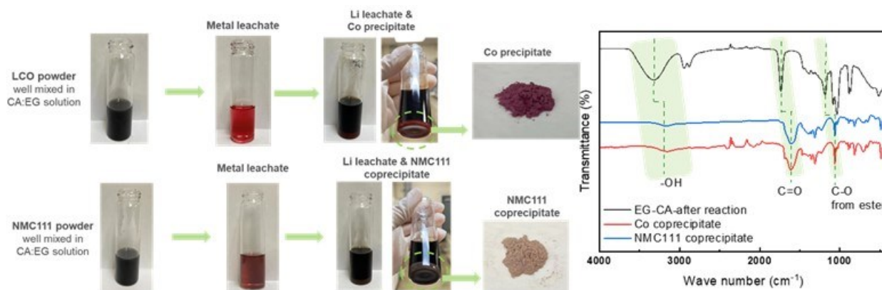
Figure III.3.44 Images of flow sheet demonstrating the process for LCO and NMC111
