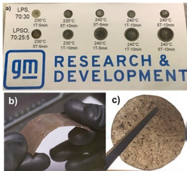
Figure XIII.4.10 a) Picture of LPS, 70:30 and LPSO, 70:25:5 reinforced pellets after hot pressing using various protocols. In general, the LPSO, 70:25:5 samples are much more deformable than the LPS, 70:30 samples. b) Picture of a hot-pressed standalone, reinforced LPSO, 70:25:5 SSE separator film. The film is flexible and translucent. c) Close up picture of the same film after being cut into a disc. The crosshatch pattern is attributed to the underlying non-woven fiber reinforcement.
