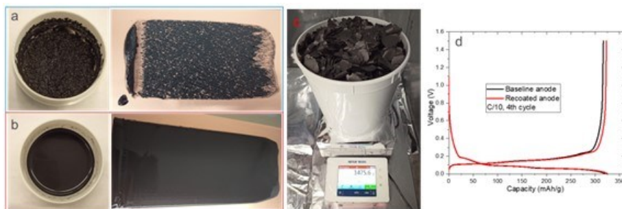
Figure III.3.10 Photos showing the slurry formed from recovered anode films using (a) KOH/EG and (b) LiOH/EG; (c) photo of ~1.5 kg recovered anode films; (d) charge/discharge profiles for the reprocessed anode in comparison with baseline anode.
