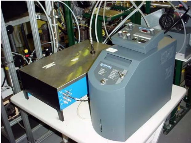
**Figure 1.** The Argonne TG-1 PM Measurement Device
