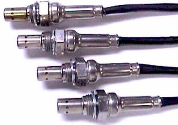
**Figure 4.** NO<sub>x</sub> Sensor Packaged Assemblies
