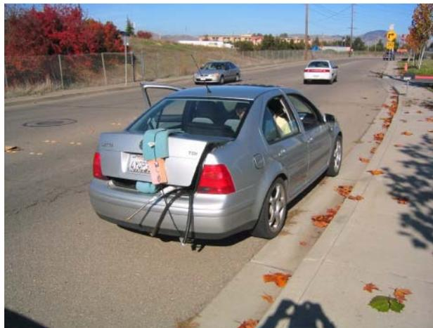
**Figure 2.** 2002 Volkswagen Diesel Jetta with the Artium LII-200™ Instrument in the Trunk
