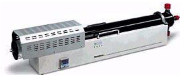
**Figure 6.** The Thermodenuder Heats the Sample to ~400°C and Absorbs the Volatiles Using Activated Carbon (The solid carbon aerosol is passed through.)
