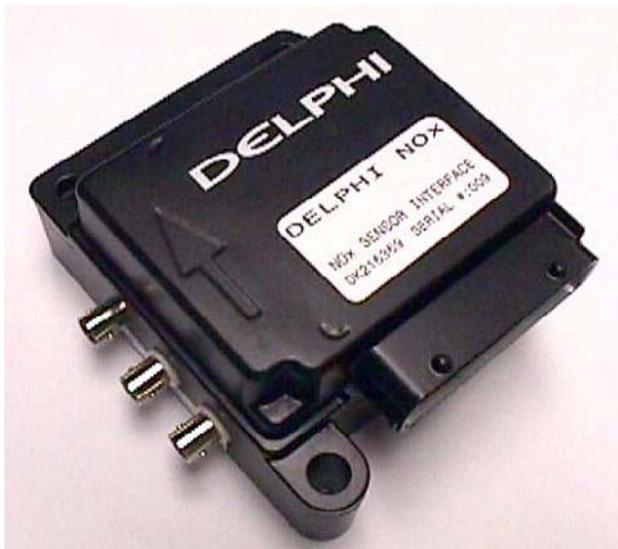
**Figure 2.** NO<sub>x</sub> Sensor Development Controller
