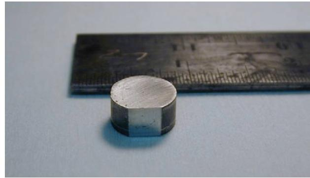
**FIGURE 2.** A 0.5" LAST ETN 121 Puck Metallized with Ni on One End and Fe on the other
