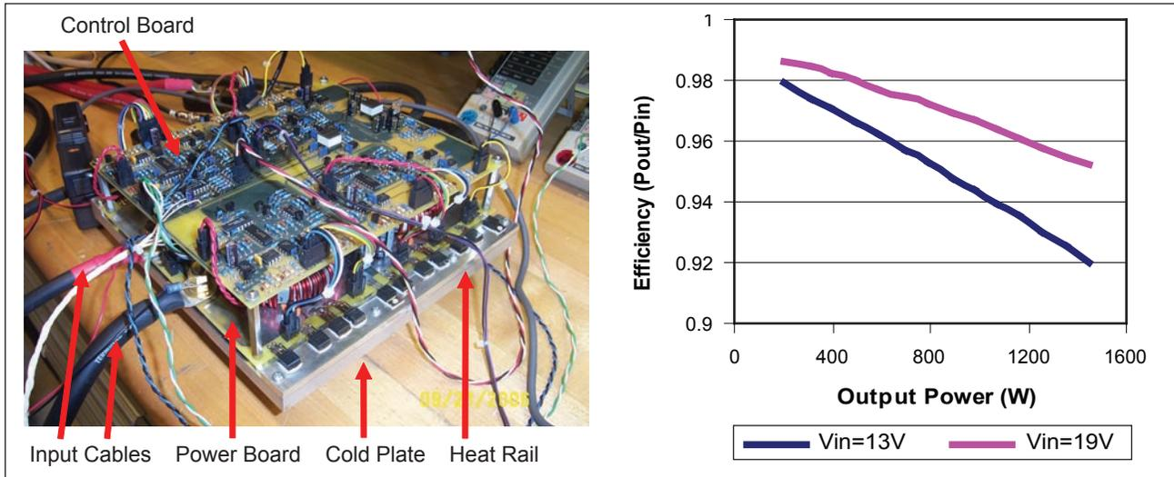
FIGURE 5. Visteon Power Converter and Test Results
