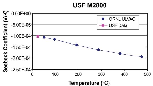
FIGURE 7. Seebeck Coefficient of a USF Clathrate Specimen
