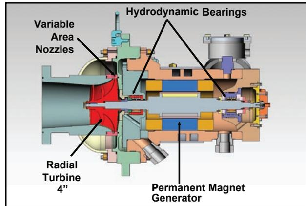
**FIGURE 2.** Proposed Turbine/Generator Design
