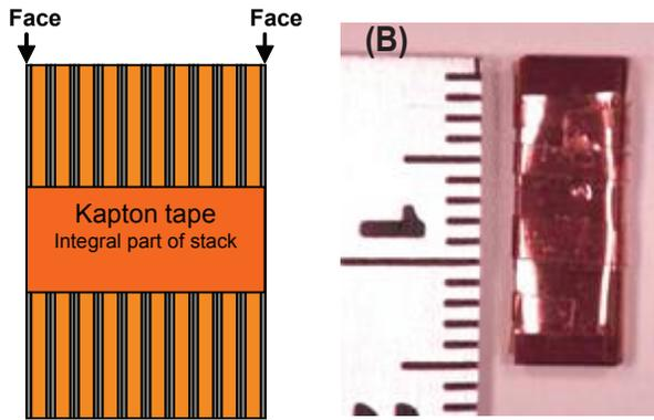
FIGURE 3. (A) Assembly and masking schematic. (B) Practice piece assembled at PNNL.
