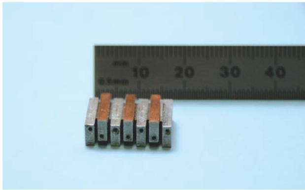
FIGURE 6. Six Bi<sub>2</sub>Te<sub>3</sub> Element Device
