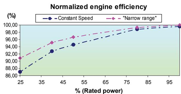
**FIGURE 2.** Engine Efficiency Comparison in "Constant" and "Narrow range" Speeds
