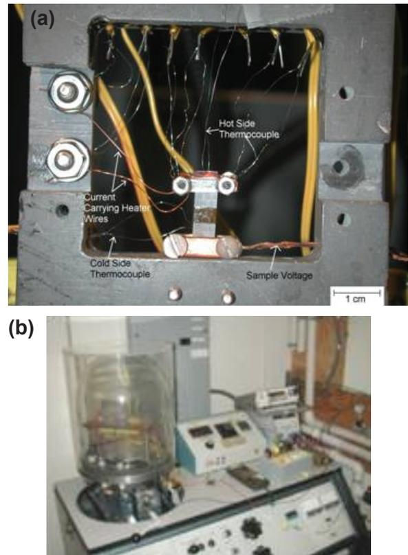
**FIGURE 2.** (A) Front view of the thermoelectric sample (P-N couple) clamped in the thermoelectric conversion efficiency rig. (B) Thermoelectric conversion efficiency rig positioned inside the vacuum chamber.
