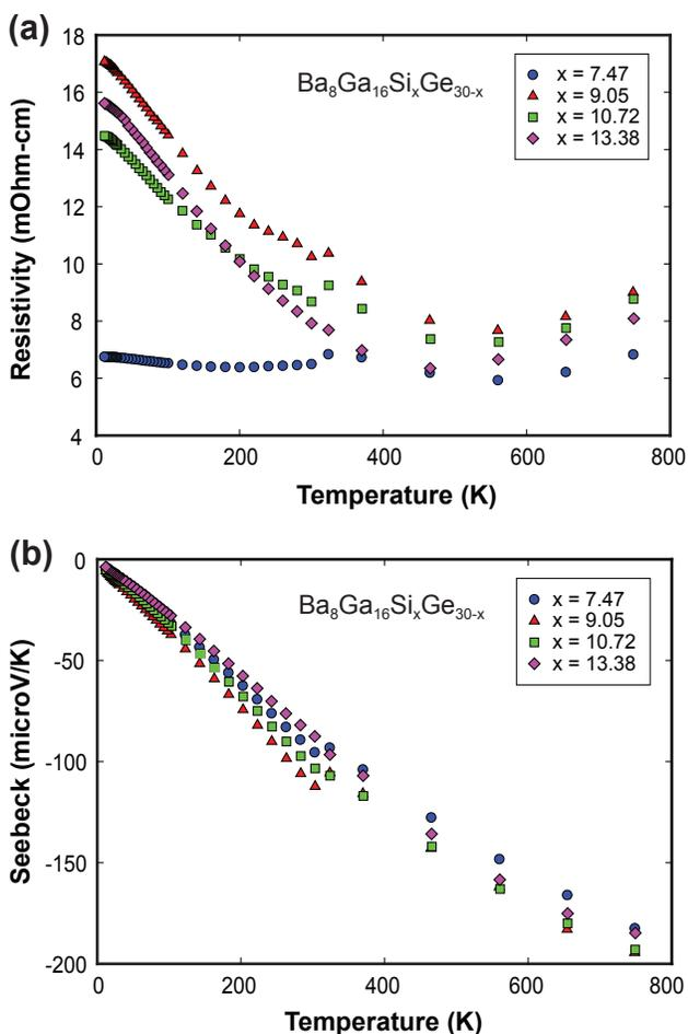
**FIGURE 8.** Low (<300 K) and High Temperature (>300 K) Transport Properties of  $\text{Ba}_8\text{Ga}_{16}\text{Si}_x\text{Ge}_{30-x}$
