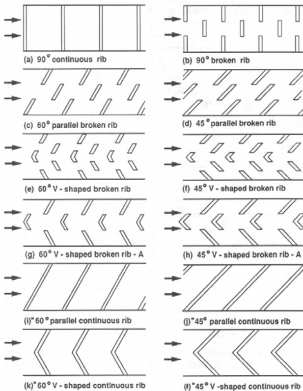
**FIGURE 3.** Examples of Heat-Transfer Enhancement Methods Involving Ribs
