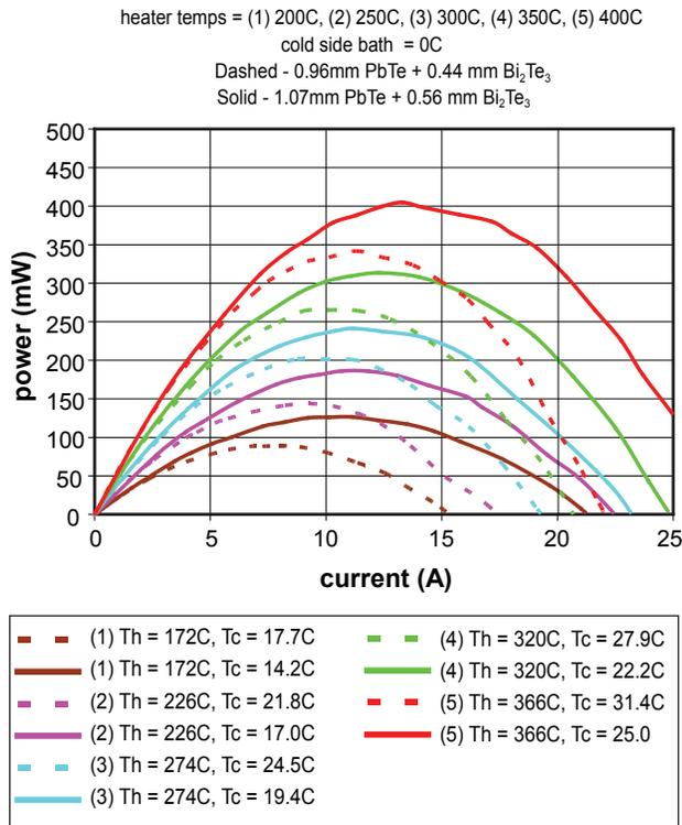
**FIGURE 8.** Power Generation Curves for Two N-Type Segmented Elements at Different Temperature Differences
