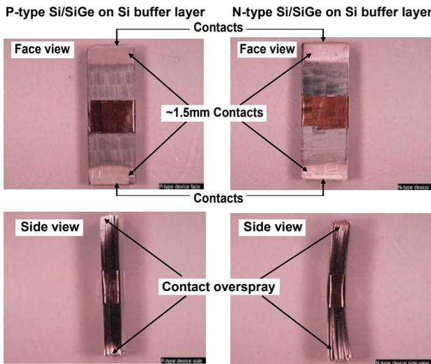
FIGURE 4. Pictures of the final, assembled P-N couple ready for conversion efficiency testing.
