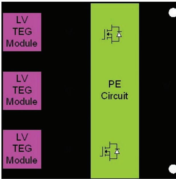
**FIGURE 1.** Using Power Electronic Circuits to Improve TEG reliability, Provide Load Matching, and Protection
