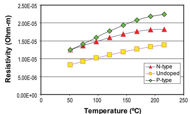
FIGURE 2. Electrical Resistivity of Marlow Elements
