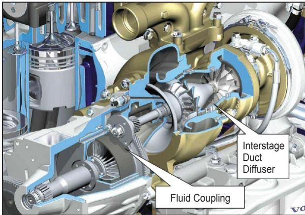
**FIGURE 1.** Close-up Showing the Turbocharger, Interstage Duct Diffuser and Turbocompound
