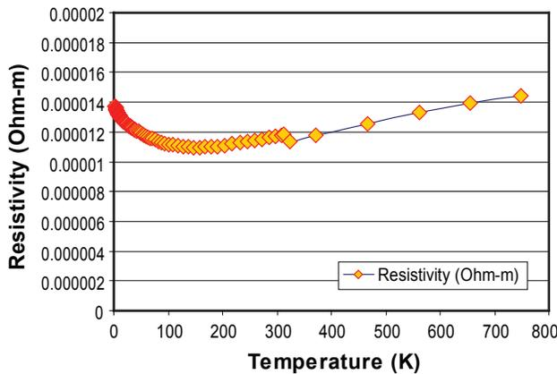
FIGURE 5. Electrical Resistivity of a GM Specimen
