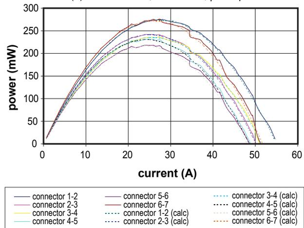
FIGURE 7. Graph Showing Power Generation Curves for Individual Bi<sub>2</sub>Te<sub>3</sub> Elements
