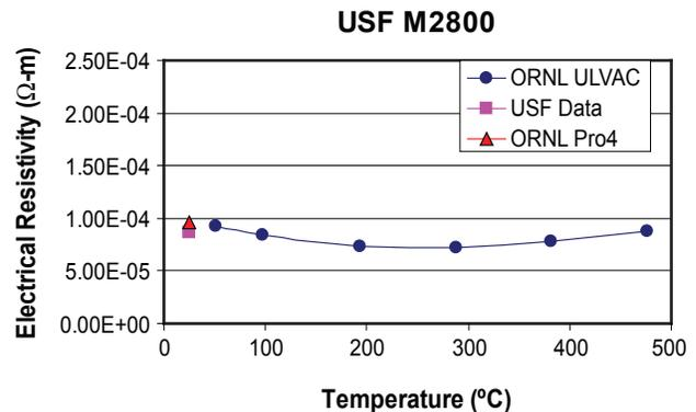
FIGURE 6. Electrical Resistivity of a University of South Florida Clathrate Specimen
