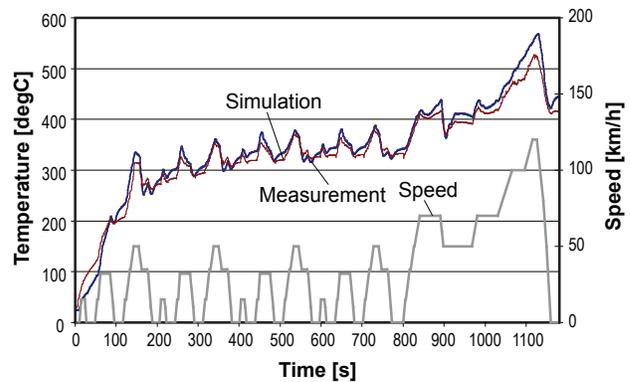
FIGURE 2. Temperature Profile of the Exhaust Gas
