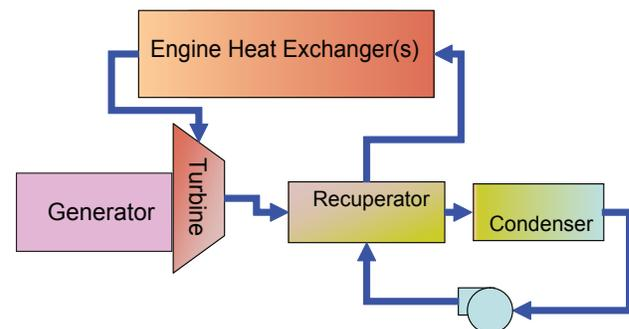
FIGURE 1. Simple Recuperated Rankine Cycle
