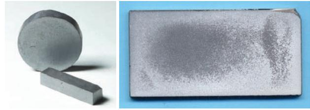
FIGURE 5. Representative bulk heterogeneous nanocomposite samples fabricated at UTRC. (A) silicon germanium, and (B) boron carbide.
