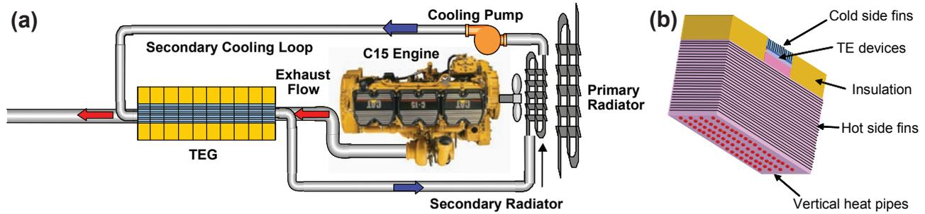
**FIGURE 1.** (A) System-level engine design, integrating a thermoelectric generator (TEG) for the purpose of waste heat recovery, with a Caterpillar C16 Engine. (B) Detailed design of the thermoelectric integrated heat exchanger (single segment).
