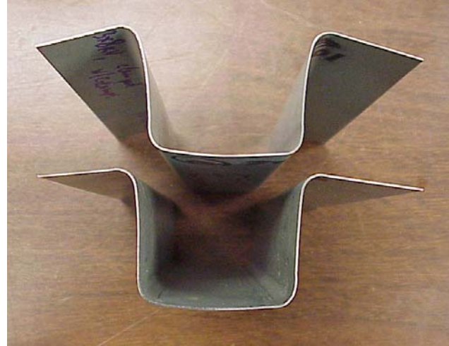
Figure 5. Improvement in springback by using EMF calibration process. (top) before, (bottom) after.
