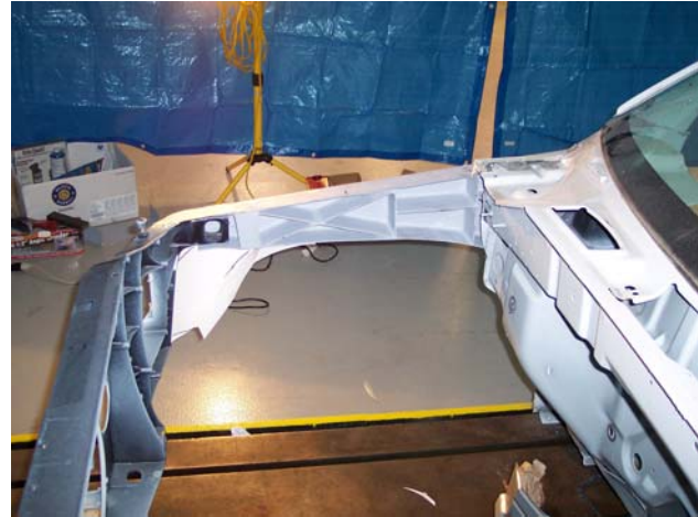
Figure 9. Cast shotgun is integrated with the body structure.
