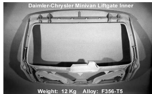
Figure 3. A single casting that replaces an assembly of 11 stampings.
