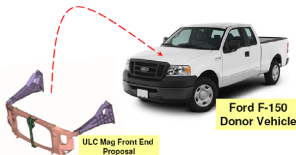
Figure 13. A demonstration front-end structure consisting entirely of large castings will replace conventional steel construction.
