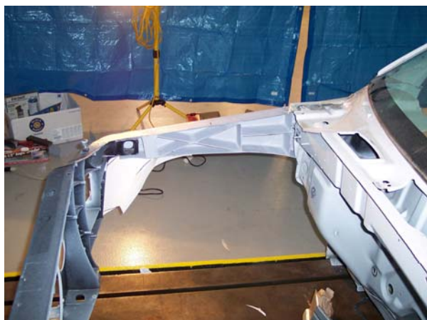
Figure 11. Shotgun will be integrated with the body structure.
