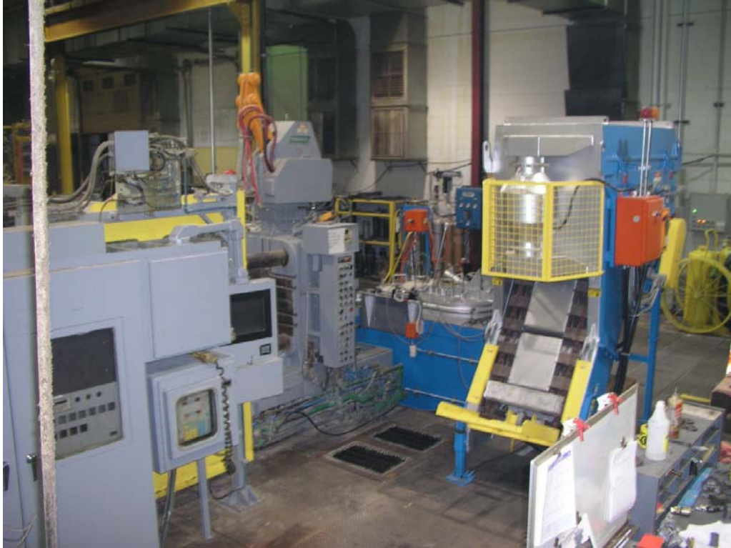
Figure 1. Squeeze-cast machine retrofitted and ready to dry-run test.
