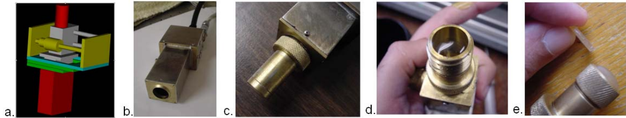
Figure 1. Mechanical drawing of the miniature scanning system (1a) encapsulated into the prototype probe housing (1b). In later prototypes, the lower section of the housing was redesigned to be much smaller for better accessibility to welds on production parts (1c). Figure 1d shows the end of the probe assembly after being filled with water, and Figure 1e shows one of the membranes tested.
