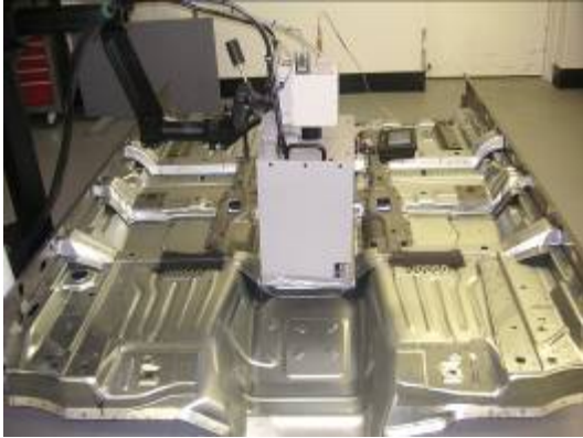
Figure 4. Pulsed-thermography inspection of a BIW truck-floor assembly.
