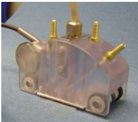
Figure 7. 17-MHz ultrasonic linear probe and custom probe holder.
