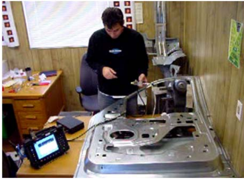
Figure 4. LBNL weld-inspection system being used to inspect a truck door provided by the Ford Motor Co. The right-hand image shows a close-up view of the portable, integrated probe positioned on a weld. The probe housing includes a miniature mechanical scanner, which allows two-dimensional images of the weld to be captured.
