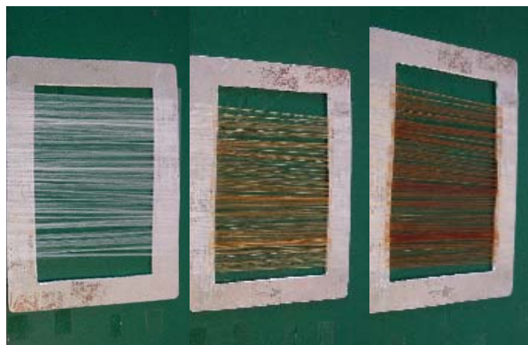
Figure 6. Virgin PAN precursor fibers, at left, exposed to increasing ultraviolet dose, at right.
