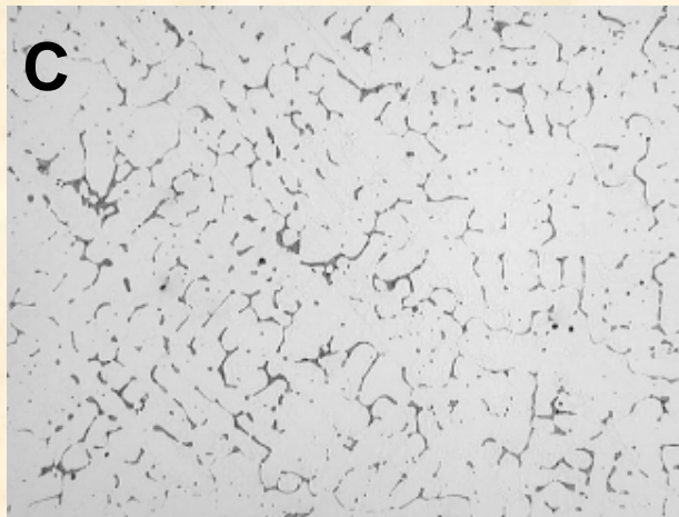
06-1799-02 Heat # M028 SFE Sand Step Cast CF8C - Plus "C" 1/2" Thick Center
