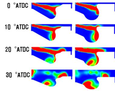
numerical simulation of combustion pattern
