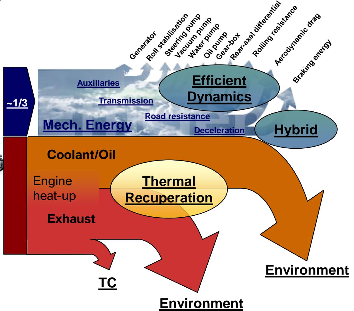
**~2/3 of the energy contained in the fuel is converted into heat**
