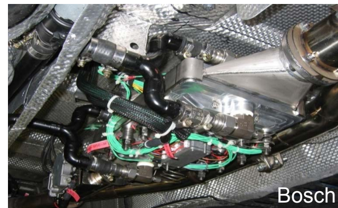
Bosch Prototype TEG in exhaust system
