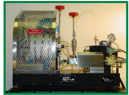
Figure 5. Ignition quality tester apparatus used to determine ignition delay for various fuels. Photo courtesy of the National Renewable Energy Laboratory.
