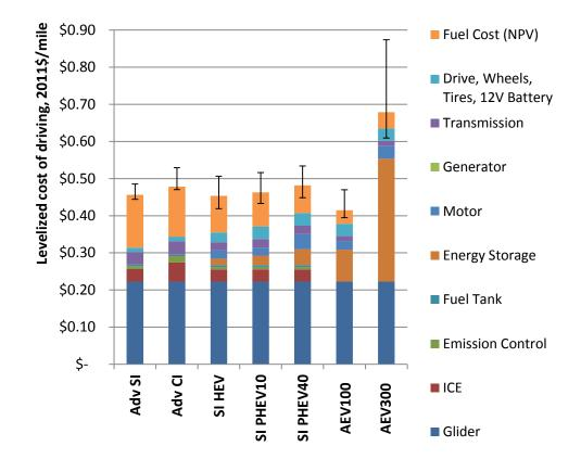
**Analysis Assumptions:** 2022 midsize vehicle, mid-case technology projection (with high and low technology sensitivities), EIA's AEO11 "High Oil" fuel prices projections for 2022 = {Gasoline \$5.12/gal, diesel \$4.76/gal, Electricity \$4.12/gge}, 14.5k miles/year, 5-year analysis period, no discounting, retail markup over manufactured cost = +50%
