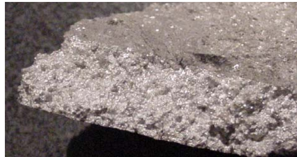
Figure 7. AZ91D fracture surface - PIVAC method.
