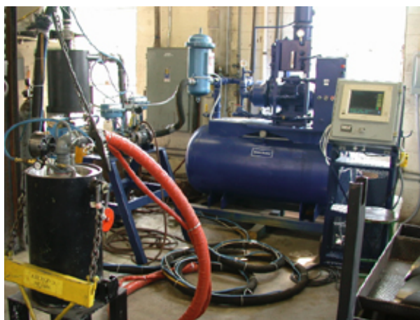
Figure 1. The Hitchiner casting system located at TTU.
