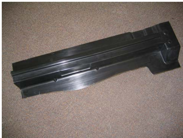
Figure 4. First “Pre-PV” part made out of Aluminum based RTM tool.
