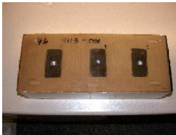
Figure 8. Hardware molded block after drilling & tapping
