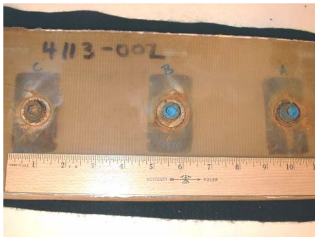
Figure 10. Hardware molded block after corrosion.
