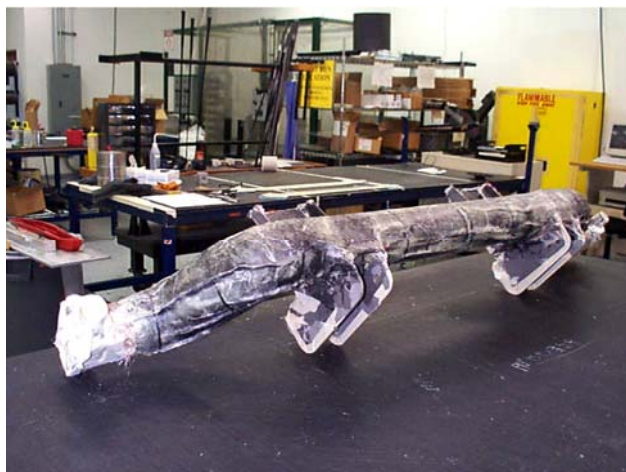
Figure 4. First composite-reinforced main support just out of cure oven, prior to any finishing work.
