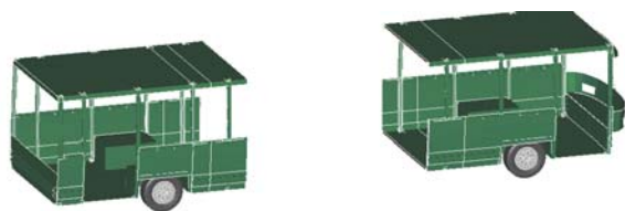
Figure 7. Non-deformable components of the FEM model.
