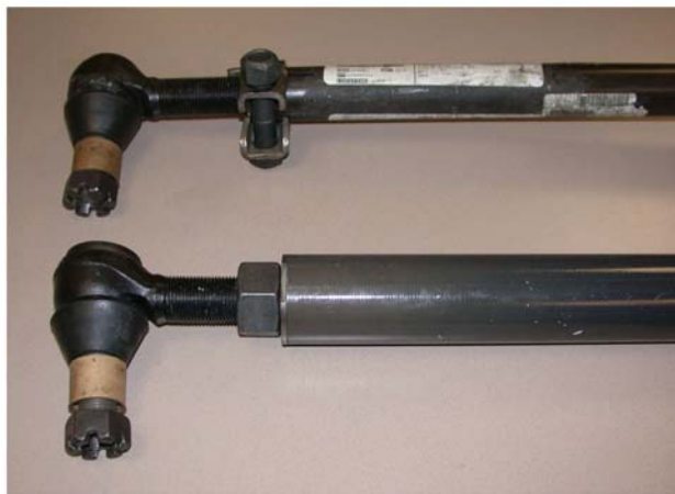
Figure 1. Typical steel and composite lateral link assemblies.
