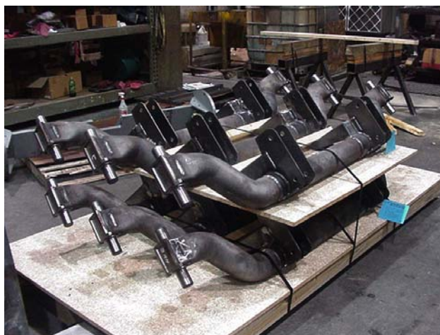
Figure 3. Prototype steel framework ready for composite fabrication.
