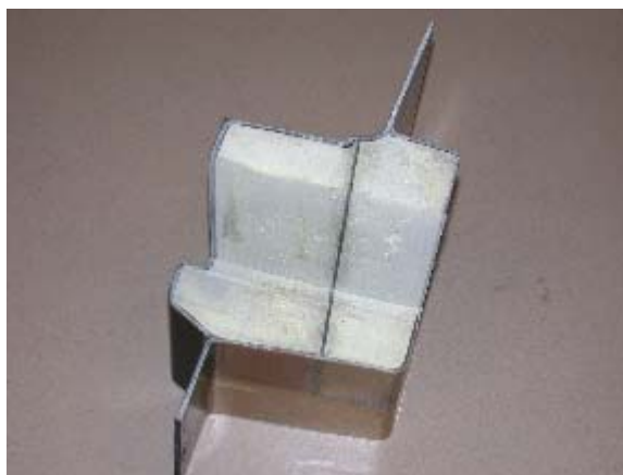
Figure 5. A cutout portion of molded “Pre-PV” part from Aluminum tool.
