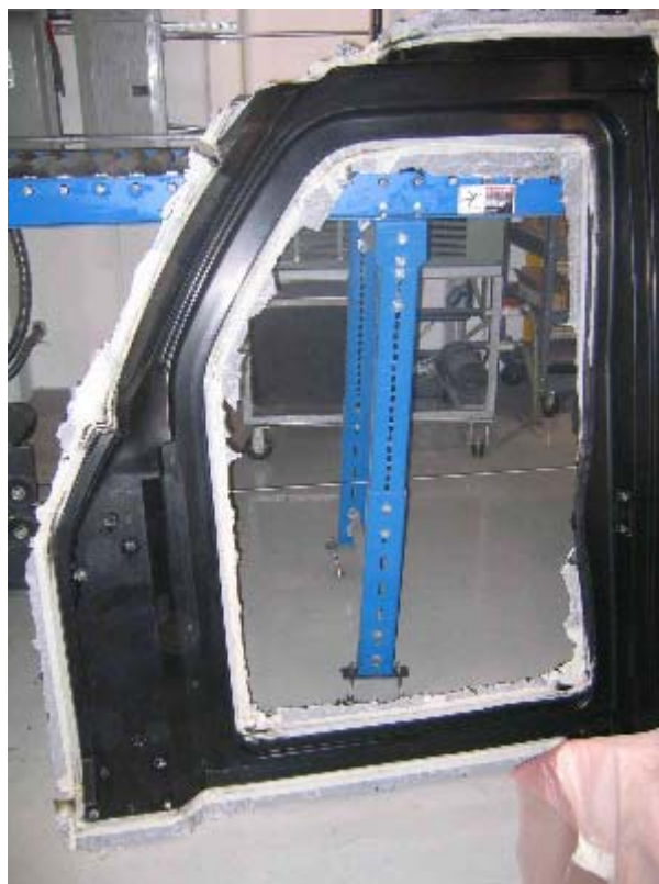
Figure 7. Exterior surface showing conductive Gel-coat.
