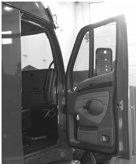
Figure 2. Prototype door assembled in Class 8 cab for functional testing.
