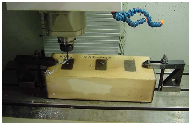
Figure 6. Drill & tap time study fixture for hardware molded test block.
