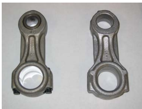
Figure 7. Machined (left) and as-cast (right) connecting rod parts.
