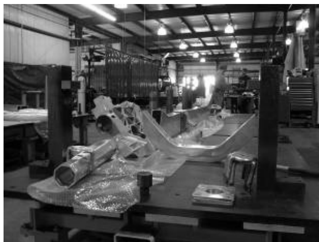
Figure 1. Next Generation frame components and assembly fixture prior to final assembly.
