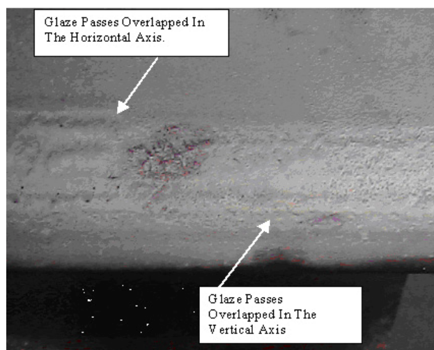
Figure 1. Dye-penetrant photograph of overlapped laser glazed tracks on 4-foot long trial rail.
