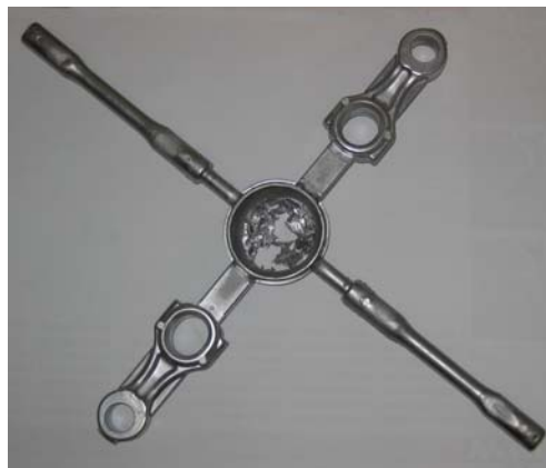
Figure 6. Typical casting from 40 shot run.
