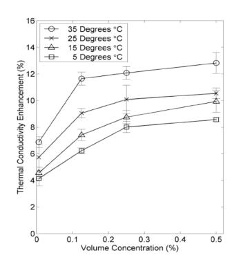
Thermal conductivity enhancement of 2 nm gold nanoparticle in water as a function of volume concentration Monodisperse gold nanoparticles with 2 nm nominal diameter were produced by a single-step water-based chemical production method. In other words, the gold nanoparticles were produced via the reduction of a gold salt by tetrakis (hydroxymethyl) phosphonium chloride (THPC). The THPC serves both as a reductant and a stabilizer that inhibits particle aggregation.
