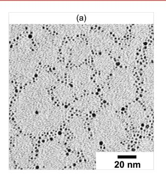
TEM micrograph of 2 nm gold nanoparticles. The number averaged diameter of the 2 nm gold nanoparticles is  $2.28 \pm 0.74$  nm.
