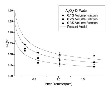
Effective viscosity enhancement of 30 nm alumina nanoparticle in water as a function of tube diameter
