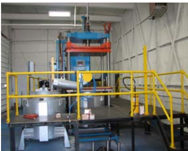
Figure 2. CMI Equipment and Engineering low-pressure casting cell.
