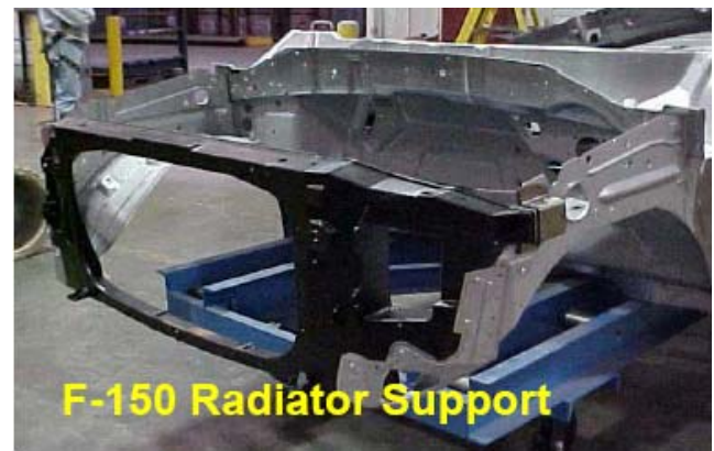
Figure 2. Cast Mg radiator support.
