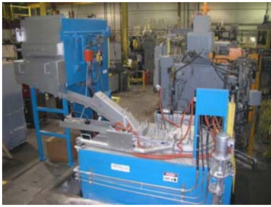
Figure 1. Contech squeeze-casting cell.
