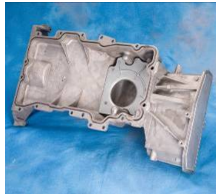
Figure 5. Finished, cast Mg structural oil pan.
