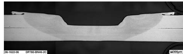
Figure 4. Optical micrograph of FSSW made in DP 790 using the BN46 stir tool.
