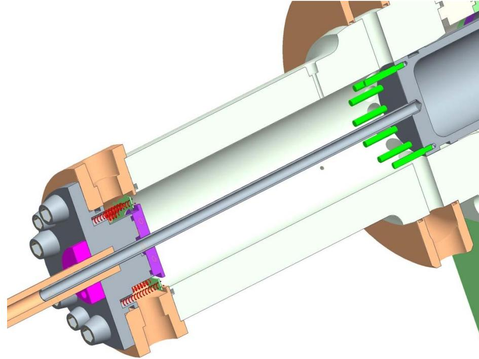
**Overview of bounce chamber design, showing injection valve at the left and vent ports to the right.**
