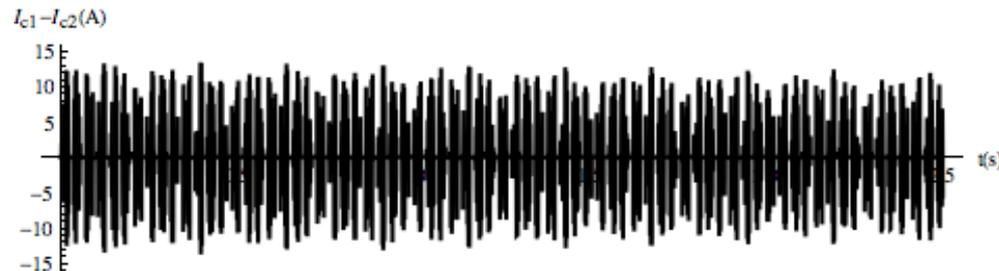
Corresponding electric power difference oscillates with the phase difference at  $\sim 14\%$  of the engine frequency. This is the mechanism by which the phases are bound in cyclic motion.
