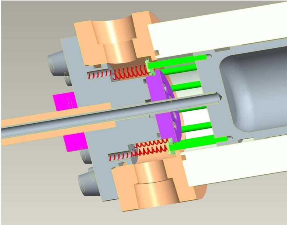
**Detail of bounce chamber air injection valve, showing piston actuation.**
