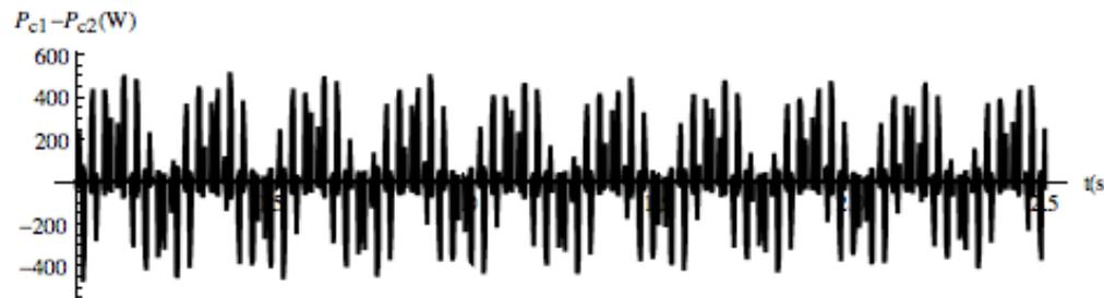
On average, Mover #2 expends 18 more Watts in friction than Mover #1, while Mover #1 produces 51 more Watts electric power than Mover #2.
