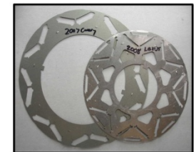
Motor rotor lamination: 2007 Camry vs 2008 LS600h
