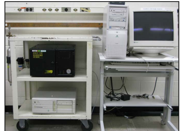
PM mass, filtration efficiency with TEOM
