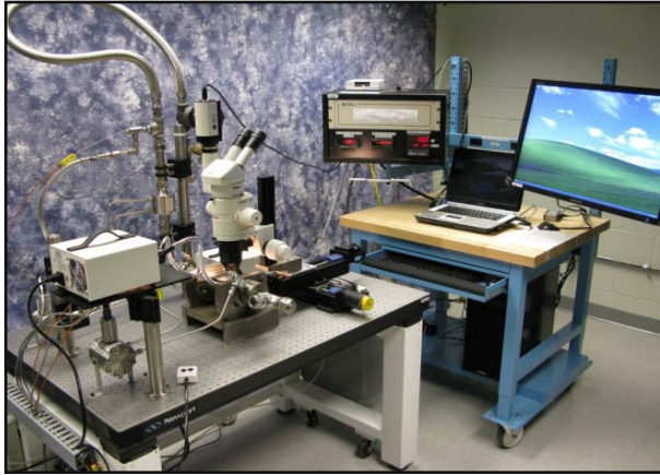
DPF experiments for filtration, regeneration, \mu -imaging
