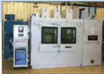
Highly Accelerated Life Test
