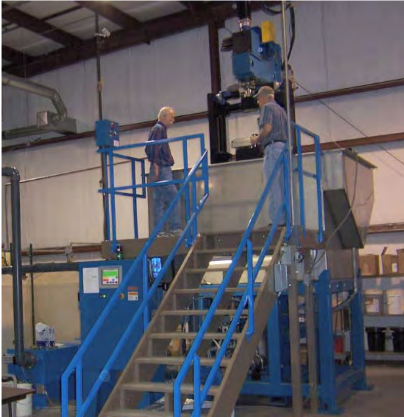
Figure 2. (A) Overview of the 20-foot tall, pilot-scale 3-DEPT™ machine. (B) Detail of the forming head of the 3-DEPT™ machine showing the forming screen for an automotive "B-pillar" (used in the Phase I project) and the four degrees-of-freedom (roll, pitch, yaw, and z-translation) that provide the unique forming capability of the 3-DEPT™ technology.
