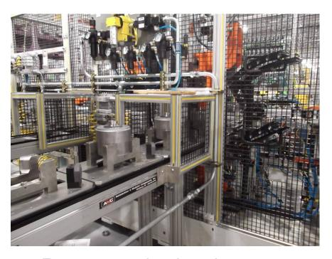
Rotors entering bearing press after magnetization
