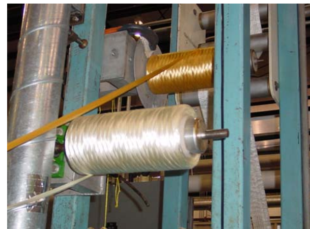
Carbon fiber precursor from modified textile PAN (polyacrylonitrile)
