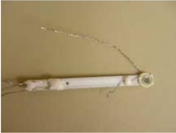
Figure 3: Photograph of LLNL HC Sensor Mounted on a HEGO Sensor
