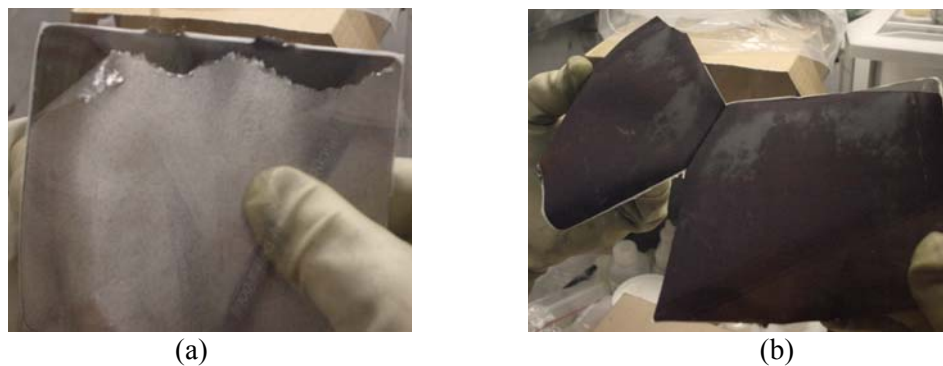
Figure 7. Post test observations on Ultralife built cell: (a) delamination of cathode from Al current collector and (b) weak adhesion & areas of stress within anode laminate.
