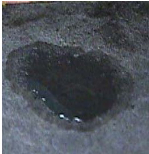
Figure 3. Water illustrates a much larger wetting angle on the carbon composite after oxidative treatment.
