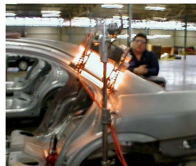
Epoxy being cured with IR heating on the Lincoln LS prototype
