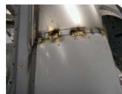
Epoxy being cured with IR heating on the Lincoln LS prototype
