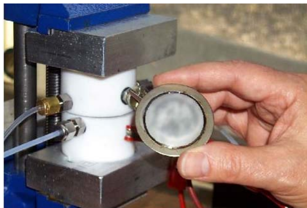
Figure 4. Teflon test cell and our membrane electrode assembly system.
