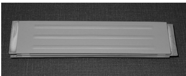
Figure 3. Sintered dielectric plates assembled in a stack with individual plates separated by alumina ceramic spacers.
