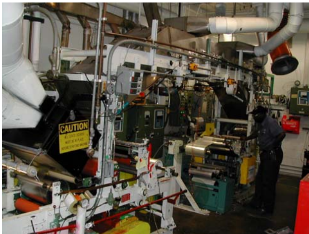
Figure 5. Brady pilot production coater with SNL film.
